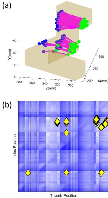
**Figure 2. Human grip point selection. (a) Thumb (green dots) and index (blue dots) contact points selected by human subjects when gripping a 3D object. For each individual grip, thumb and index fingers are connected by magenta vectors. (b) The same grip point couples from (a) projected as yellow diamonds onto the penalty map computed for the specific 3D object shown.**
