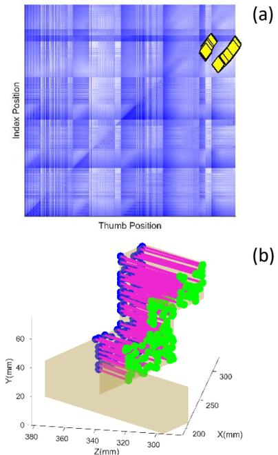
**Figure 3. Grip locations selected by the model. (a) Grip point couples (yellow diamonds) selected from the two deepest local minima of the penalty map. (b) Same thumb (green dots) and index (blue dots) grip point couples projected onto the 3D object. For each individual grip, thumb and index fingers are connected by magenta vectors.**
