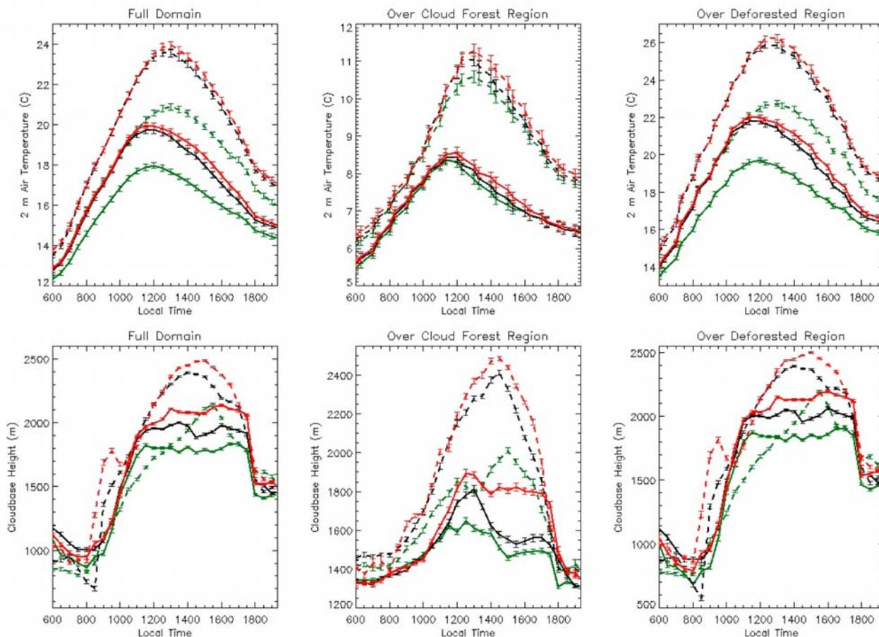
**Figure 4.** Impact of atmospheric information on simulating (top) 2 m air temperature and (bottom) cloud base heights. Solid lines are associated with simulations done with special radiosondes, whereas dashed lines are for simulations done with standard atmospheric information. Green denotes pristine/forest conditions, black denotes current conditions, and red denotes future deforested conditions. The error bars are associated with the standard error in each case.
