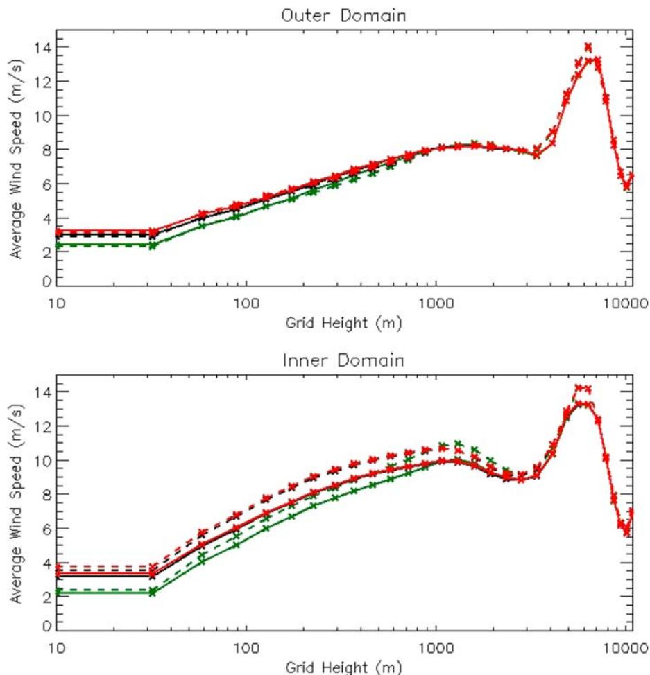
**Figure 6.** Variation of domain-averaged wind speed with height for all special atmosphere simulations for outer coarser domain and for the entire simulation time. The initial increase of wind speed with height decreases at around 3.5 km, and then it rapidly increases. This is associated with the trade wind inversion found in this region.
