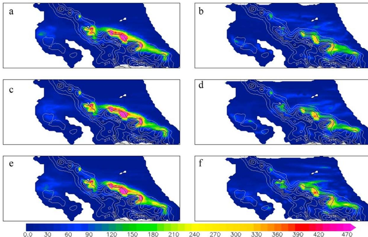
**Figure 3.** Simulated precipitation (mm) over the outer grid over the simulation period for six different models to estimate the importance of special radiosondes: (a) F\_SPECIAL run, (b) F\_STANDARD run, (c) C\_SPECIAL\_ATM run, (d) C\_STANDARD\_ATM run, (e) D\_SPECIAL run, and (f) D\_STANDARD run.
