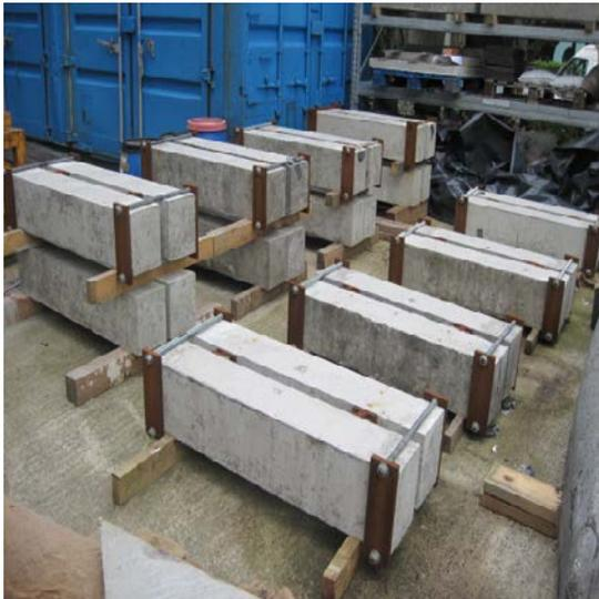
Figure 2. Test beams under sustained loading.
