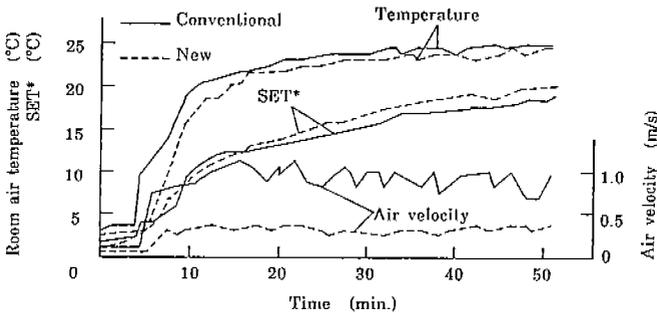
Fig.9 Variation of air temperature, SET\* and air velocity around the remote controller
