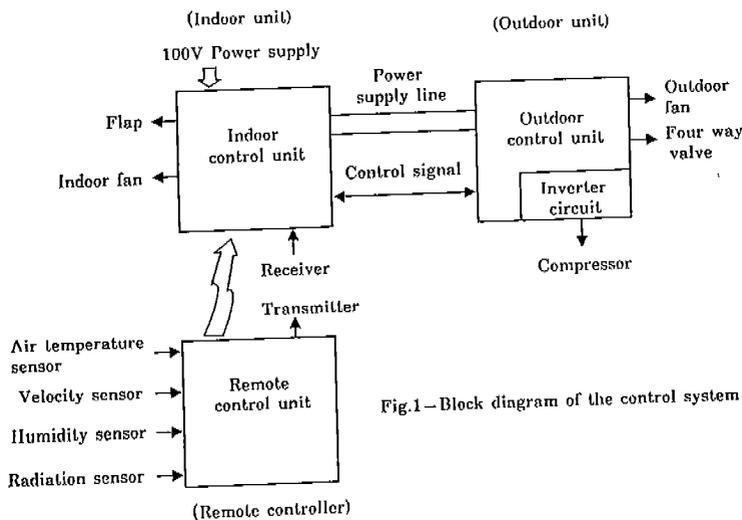
Fig.1—Block diagram of the control system
