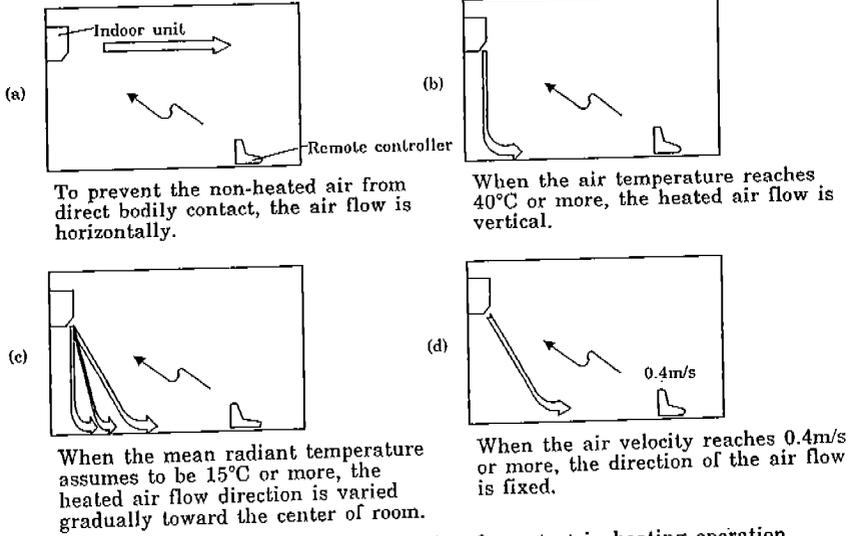
Fig.8—The directional control of air flow from start in heating operation.
