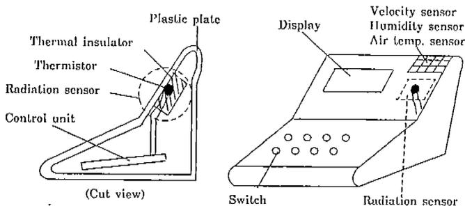
Fig.2—Configurations of radiation sensor and remote controller
