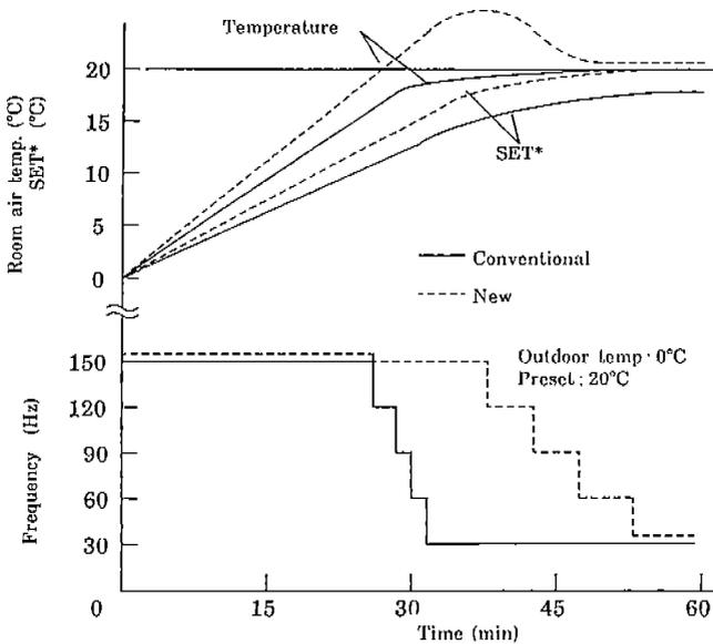
Fig.7- Comparison of results controlled by room air temperature and SET\*
