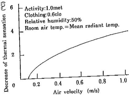
Fig.5 - Influence of air velocity for thermal sensation
