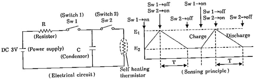
Fig.4 - Schematic diagram of electrical circuit and sensing principle in velocity sensor
