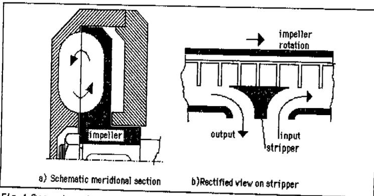
Fig. 1 Geometry of peripheral pump
