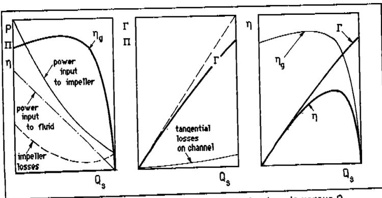
Fig. 5: Theoretical powers, losses and efficiencies trends versus  $Q_s$
