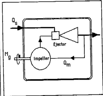
Fig.2 Turbomachine-ejector system
