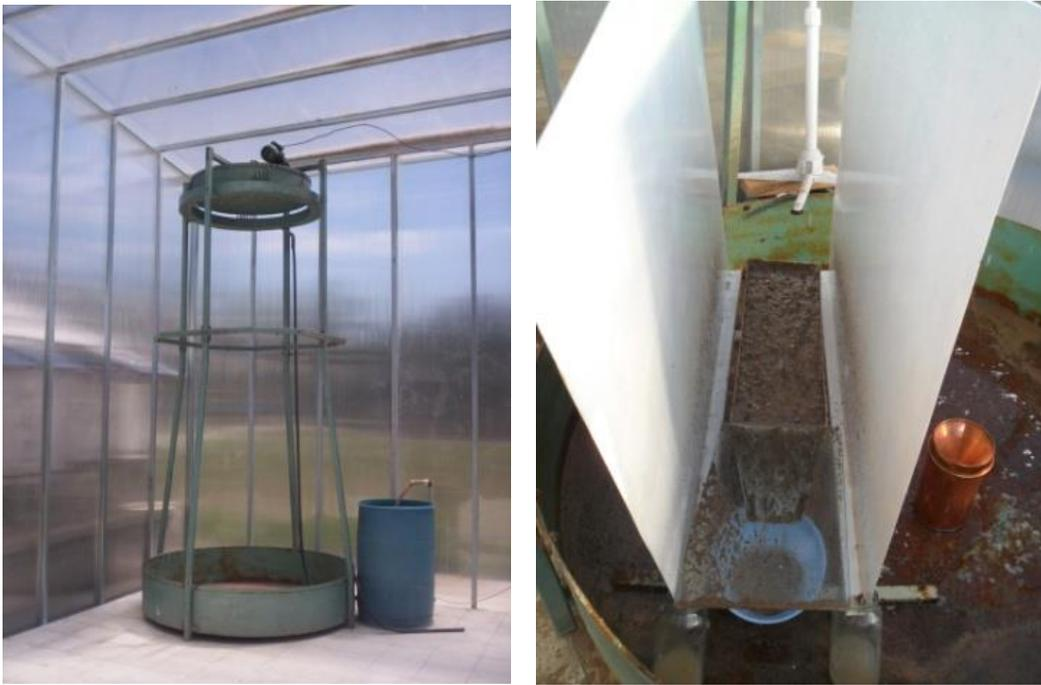
**Figure 1.** Rainfall simulator (left) and experimental setup in laboratory (right).
