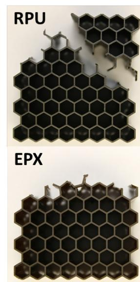
Figure 2: (Left) Example test data showing stress vs strain for two parts compressed in the X2 direction. The parts are printed from either EPX or RPU, with  $t/l = 0.20$  and relative density of 0.23. (Right) Post compression samples in RPU and EPX.
