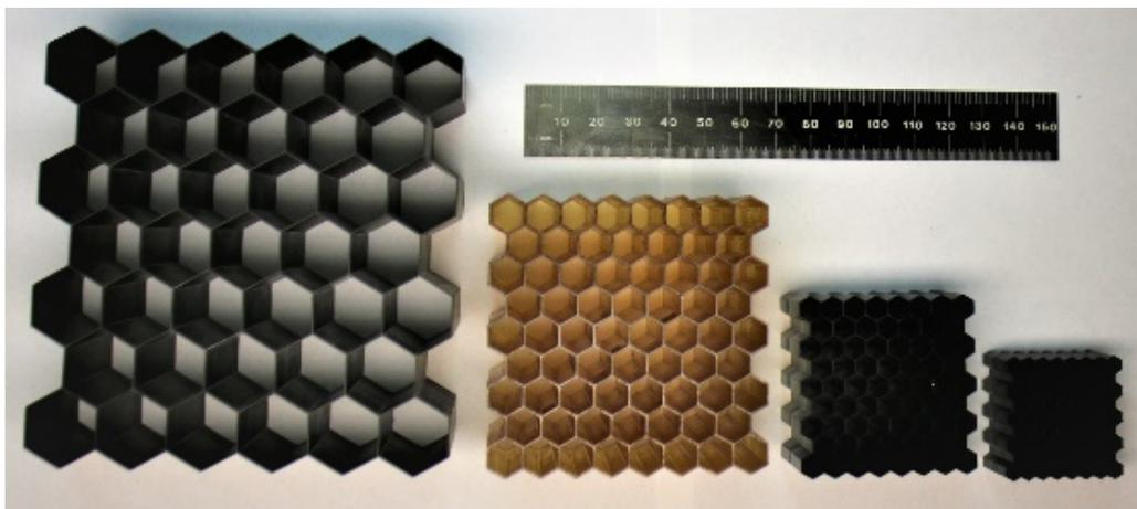
Figure 1: Hexagonal lattices printed using CLIP in four different materials (left to right) EPX, CE, RPU, and FPU at relative densities of 0.06, 0.12, 0.12, and 0.23 respectively. The ruler shows millimetres.
