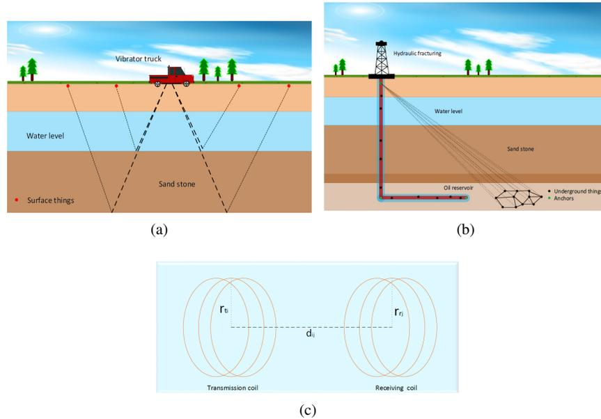
Fig. 10.3: Communication Technologies in IOUT: (a) Acoustic-based IoUT, (b) EM-based IoUT, (c) Schematic of MI communication link [114]
