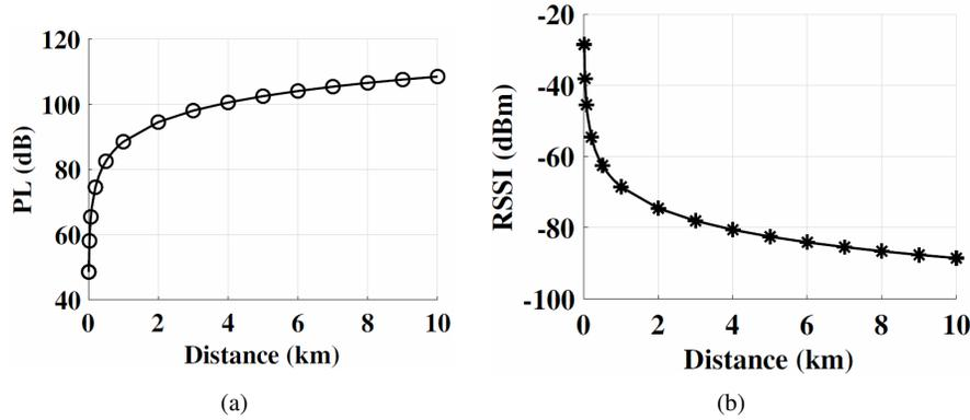
Fig. 10.8: (a) Effect of distance on path loss [44], (b) Effect of distance on RSS [44]
