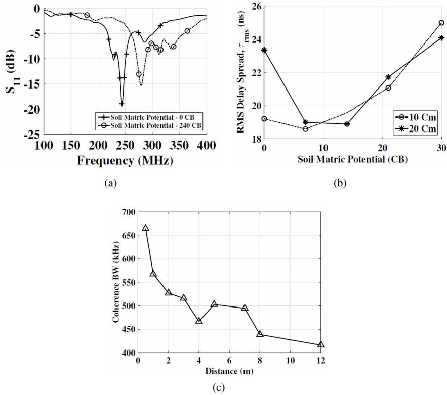
Fig. 10.11: (a) Effect of soil moisture on antenna return loss at varying frequencies and fixed depth of 40cm in sandy soil [139], (b) Effect of soil moisture on RMS delay spread at T-R separation distance of 50cm and two depths of 10cm and 20cm [139], (c) Effect of T-R separation (distance) on coherence bandwidth at fixed depth of 20cm in silty clay loam soil [139]
