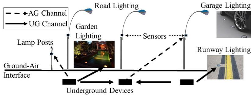
Fig. 10.4: IOUT-based smart lighting architecture [52]
