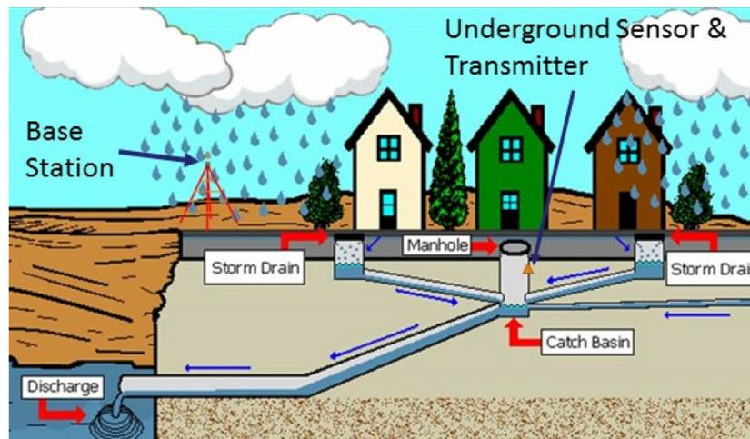
Fig. 10.6: IOUT-based Urban underground infrastructure: Smart wastewater system [44]
