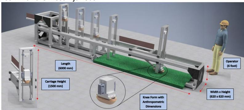
**Figure 1:** Novel test rig to assess potential for skin injuries on Rugby Turf.
