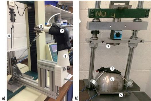
Fig. 1: ISO 20320:2020 performance test setups (a) limitation of wrist extension test (b) impact performance test. 1- Polyamide hand and wrist surrogate, 2 -wrist protector, 3 - steel rods to apply the load, 4 - displacement to generate torque in surrogate wrist, 5 - load cells, 6 - hemispherical dome, 7 - guided falling mass
