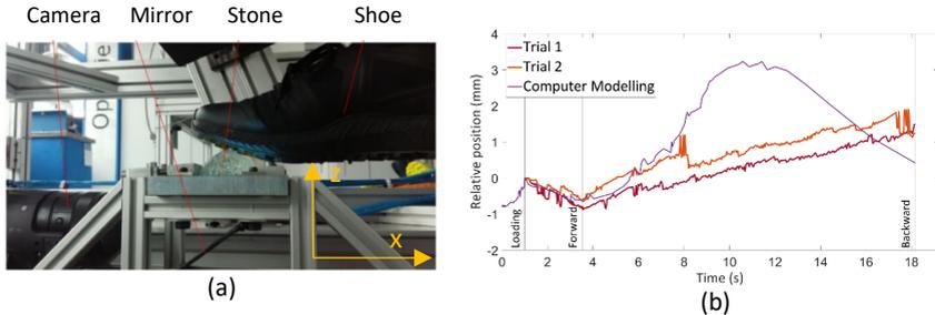
**Fig. c:** (a) Experiment setup installed in the TrakTester; (b) Relative movement of the tip of the stud in relation to the shoe sole position
