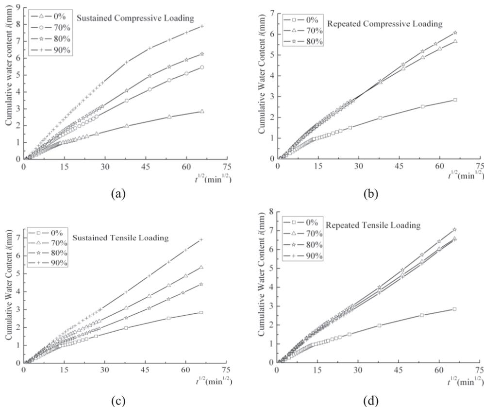
Figure 4. Effect of load level of different patterns on cumulative water absorption. (a) Sustained compression. (b) Repeated compression. (c) Sustained tension. (d) Repeated tension.
