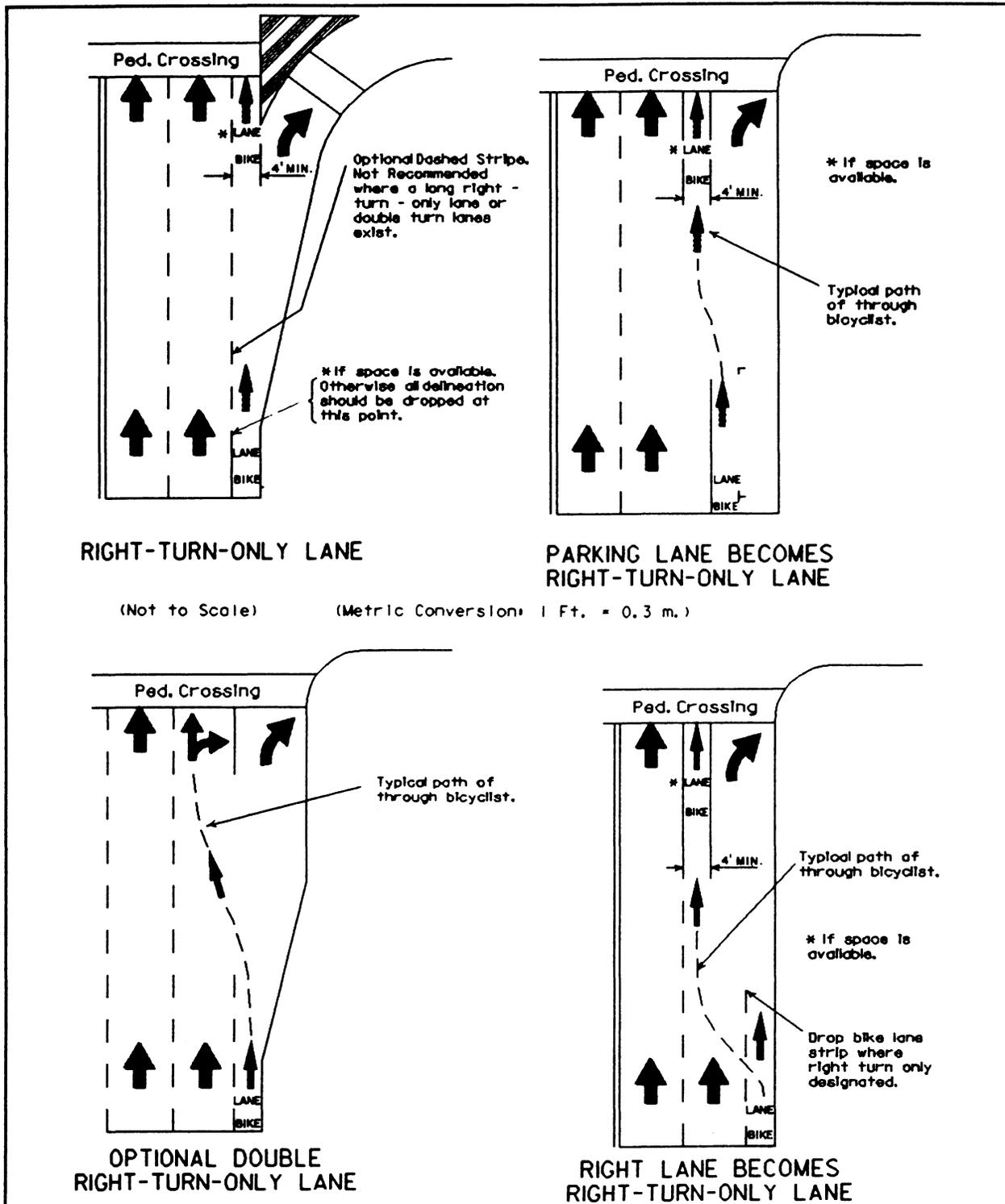
**Figure 3: Bicycle Lane Treatments at Intersections with Right Turn Lanes**
