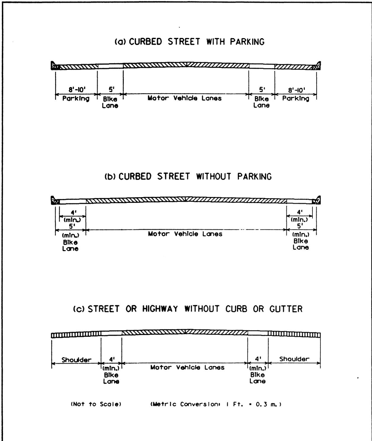
Figure 2: Examples of Typical Cross Sections for Bicycle Lane Designs
