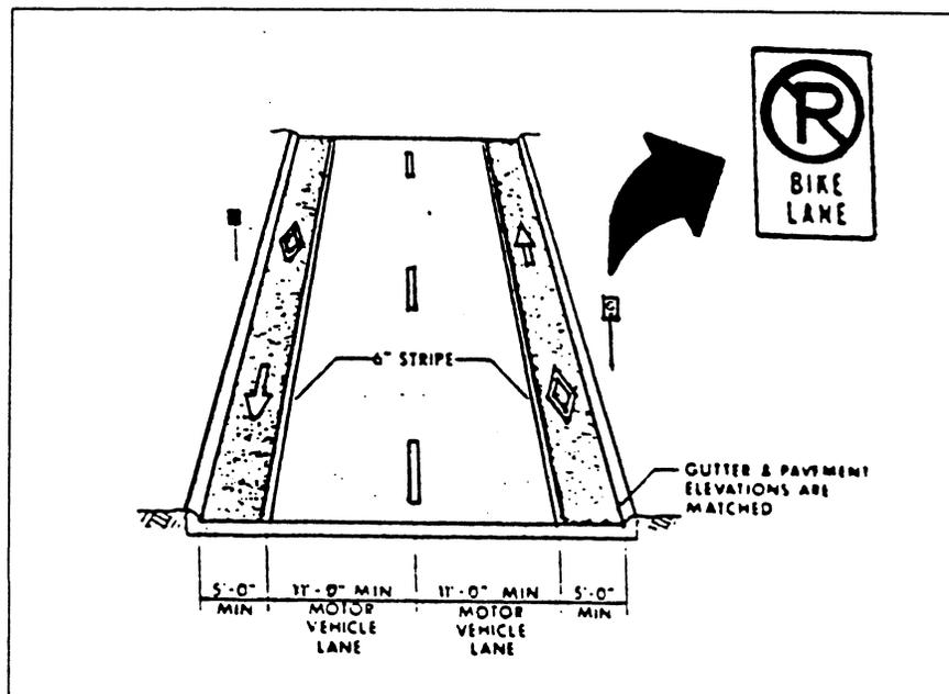
**Figure 1: Typical Road Design with Bicycle Lanes**
