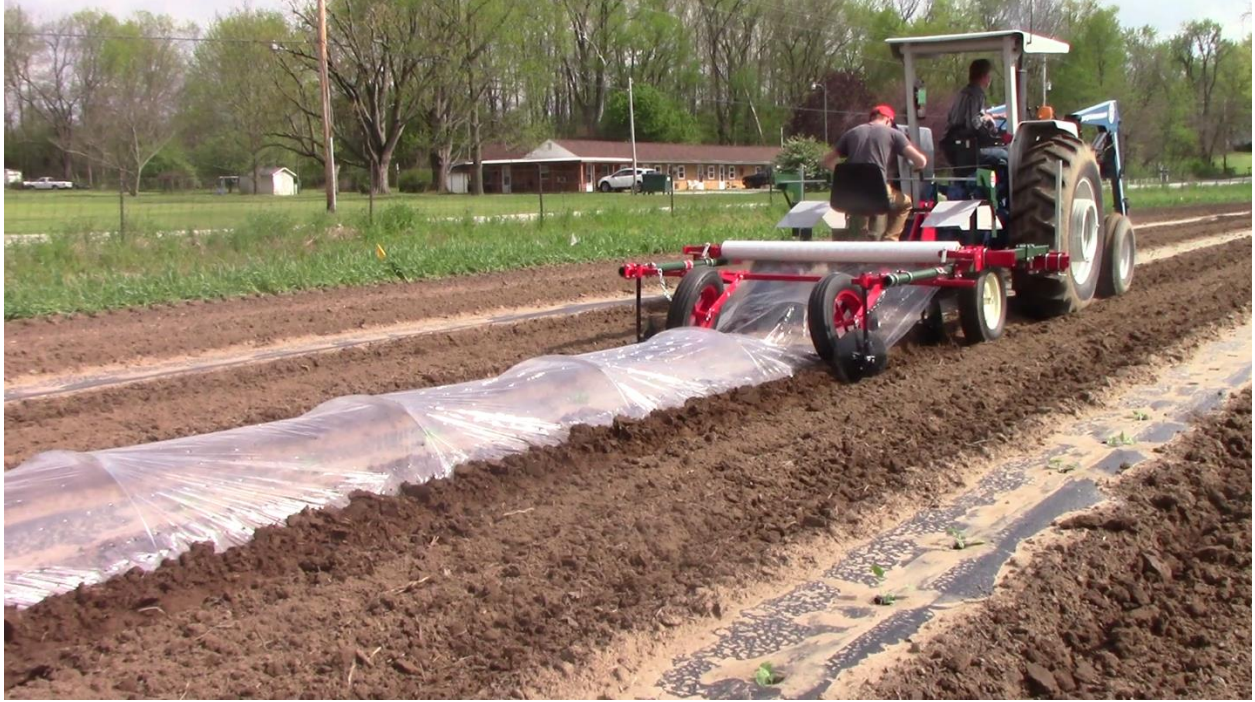
Figure 1. Low tunnel covered with 1 mil perforated row cover was installed using a mechanical transplanter low tunnel layer on 24 Apr. 2020.
