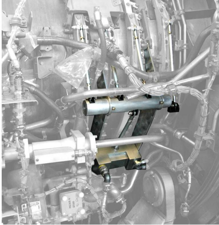
Figure 3: Variable stator vane actuator control system project
