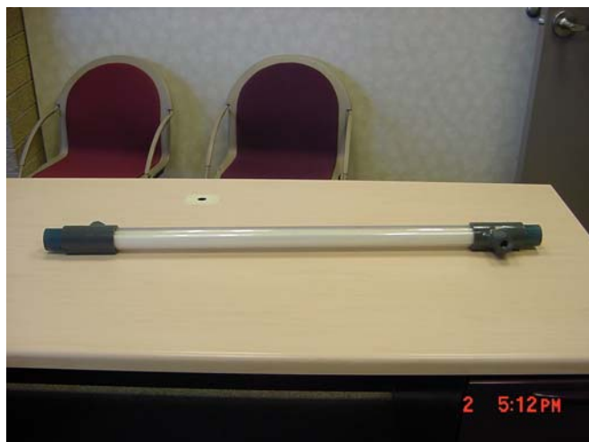
Figure 1. Picture of the housing unit for the woven fabric membrane meant to filter out bacterial cells and other organics
