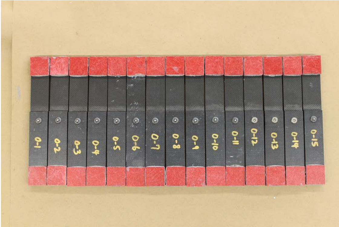
Figure 7. 15 conventional hybrid joint test specimens.
