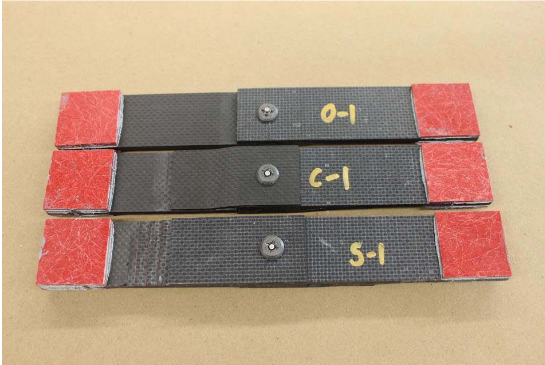
Figure 5. A top view of the three different types of hybrid joints.
