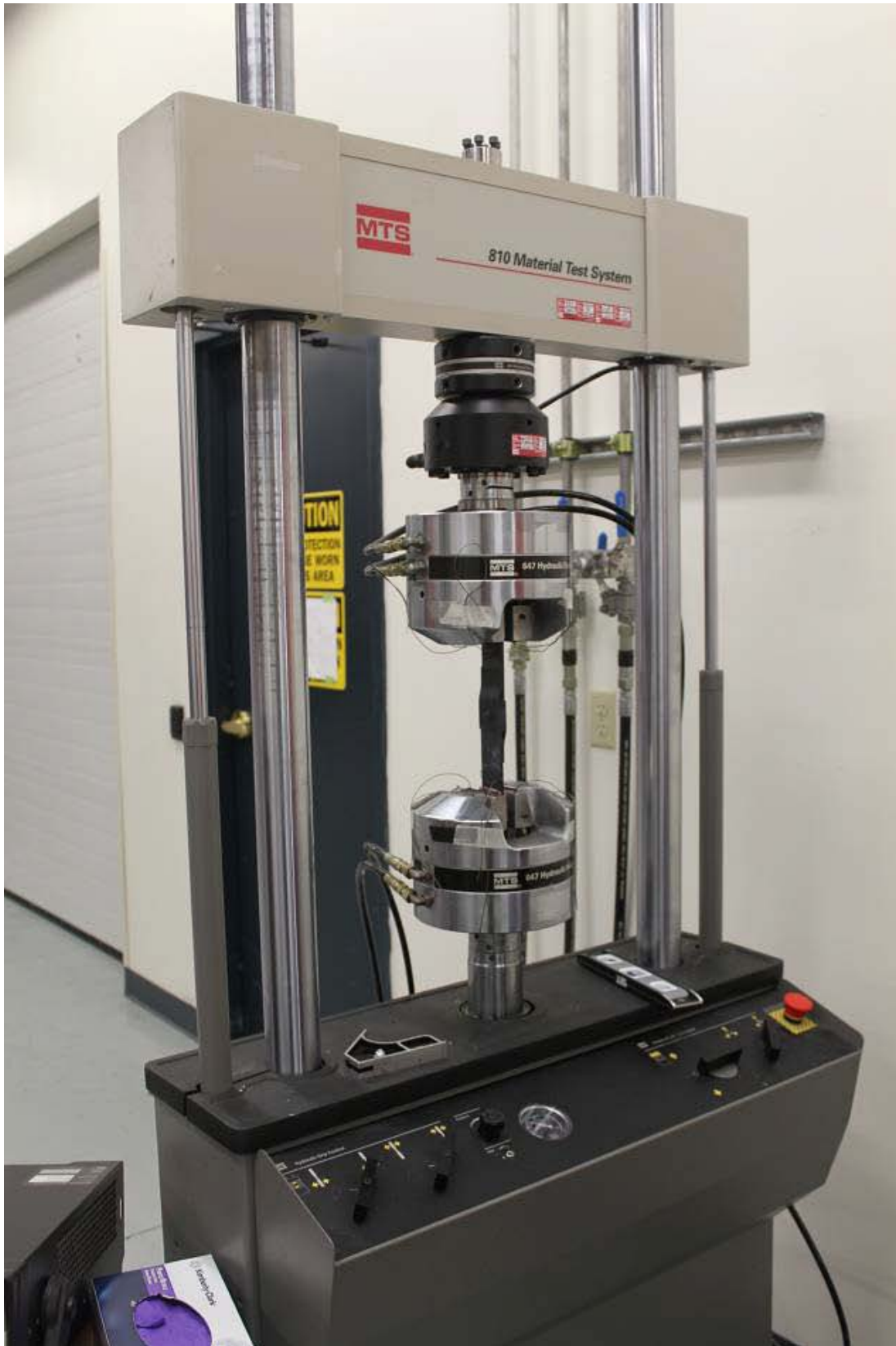
Figure 6. MTS Systems Corporation tensile tester with a 22 kip ( \pm 100\text{kN} ) load cell.
