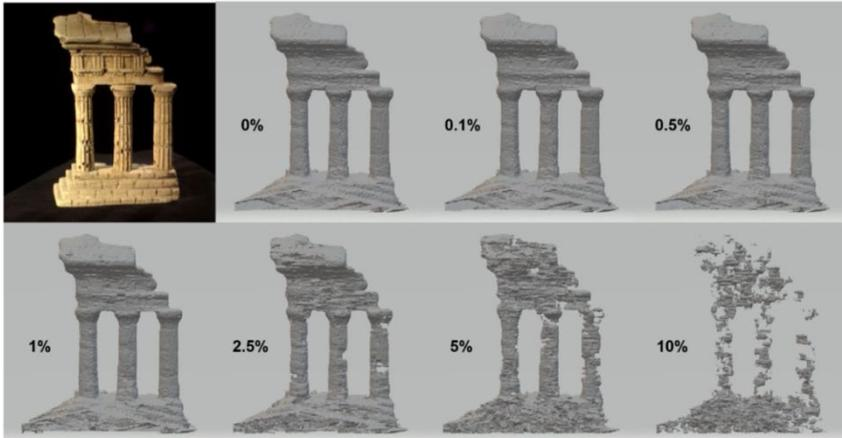
Fig. 1: *Qualitative interpretation of the effect of silhouette accuracy on visual hull accuracy. The top left image is one of the images in the TempleRing dataset. Every other image was obtained by reconstructing a visual hull from the TempleRing dataset using silhouettes that were altered by a percentage indicated by the number reported next to each figure.*
