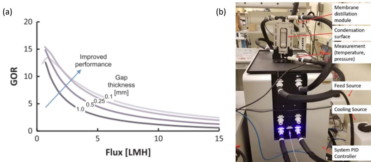
**Fig.2** (a) Energy efficiency described by the Gained output ratio (GOR) versus permeate flux for varying air gap thickness [10]. It shows that the optimal gap thickness is below 0.25mm which is far less than the thickness possible with the current filmwise condensation regimes in AGMD. (b) Membrane distillation setup with flexibility to change air gap thickness, inclination angle and condensing surfaces.
