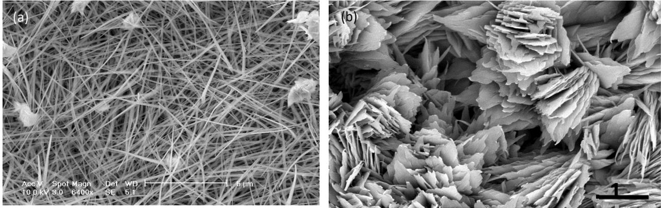
**Fig 3.** SEM images of (a) CuO nanowires grown on condensing surface before coating it with PDMS, the final step in making it superhydrophobic; scale bar = 5 μm (b) Slippery liquid infused porous surface (SLIPS); scale bar = 1 μm. The nano-structures on both the surfaces are different resulting in different surface characteristics.
