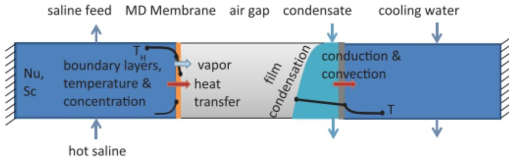
**Fig.1** Schematic of air gap membrane distillation (AGMD) computational cell for numerical modeling that includes temperature variations in the concentration boundary layers, flow directions of vapor, heat, feed, cooling water and condensate [10]. Several hundred such cells are used to model a full membrane module.
