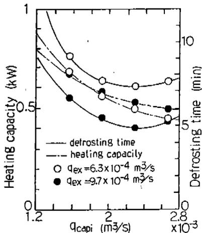
Fig. 7 - Heating capacity and defrosting time vs.  $q_{capi}$
