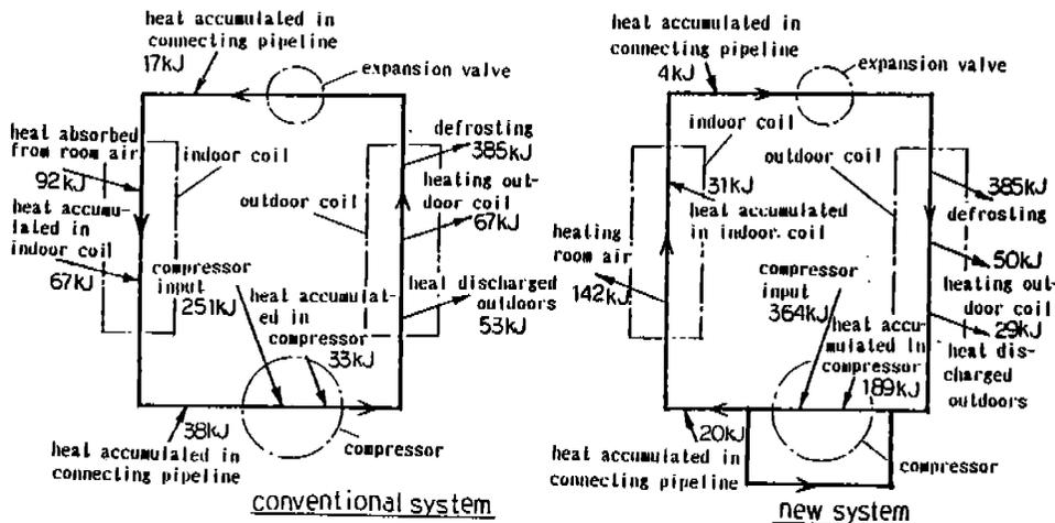
Fig. 6 - Heat balance during defrosting
