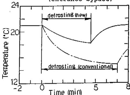
Fig. 13 - Changes in mean indoor temperature during defrosting
