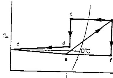
Fig. 3 - Pressure-enthalpy chart of the refrigeration cycle
