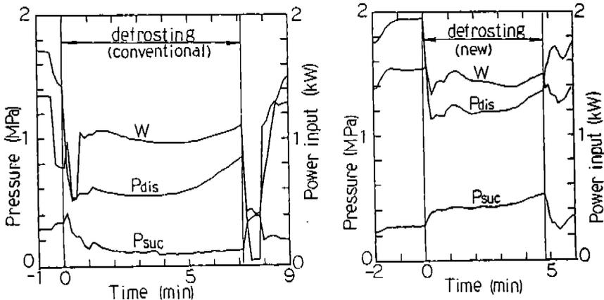
Fig. 5 - Power input and pressure changes during defrosting
