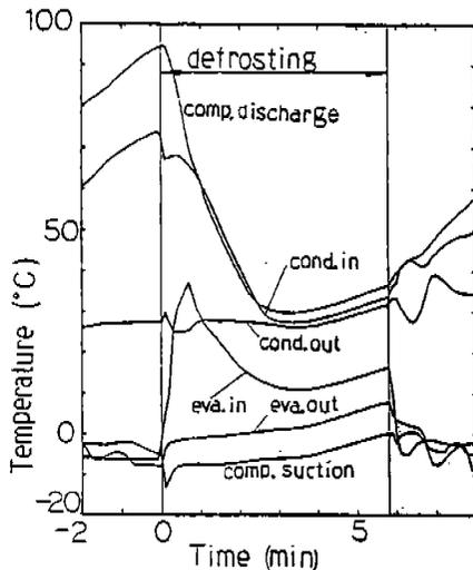
Fig. 11 - Temperature changes during defrosting (entrance bypass)
