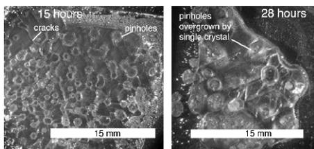
Figure 3. The effect of growth time on AlN crystal morphology at  $T_G=1930^\circ\text{C}$  and a source-to-seed distance of 10 mm. Left: AlN single crystal, 200-300 mm<sup>2</sup> large and 300-350  $\mu\text{m}$  thick, after 15 hours of growth; Right: AlN single crystal, 200-300 mm<sup>2</sup> large and 650-700  $\mu\text{m}$  thick, after 28 hours of growth.
