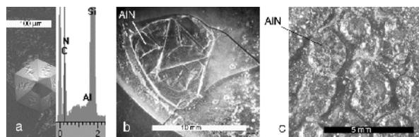
Figure 2. The effect of temperature on AlN growth observed in three samples: a) SEM image of the hexagonal features grown at  $T_G=1820-1830^\circ\text{C}$ , EDX of these features ( $\text{AlN}_x\text{SiC}_y$ ); b) AlN single crystal growth at  $T_G=1870-1880^\circ\text{C}$ ; cracks due to thermal and mechanical stresses are evident; c) colorless and transparent AlN islands with flat c-faces grown at  $T_G=1920-1930^\circ\text{C}$ .
