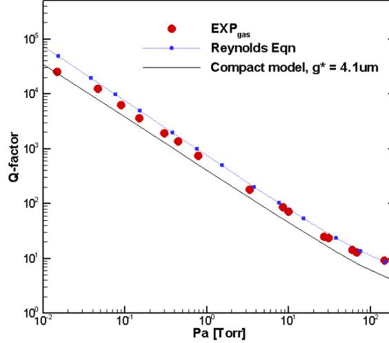
Figure 6. Comparisons of predictions by the ESBGK-based compact model and experimental data in reference,<sup>1</sup>  $L = 193\mu\text{m}$ ,  $b = 154\mu\text{m}$ ,  $g_0 = 4.1\mu\text{m}$ ,  $t = 5.7\mu\text{m}$ ,  $\rho_s = 19.3e+3 \text{ kg} \cdot \text{m}^{-3}$ ,  $E = 78\text{GPa}$ , Mode-1.
