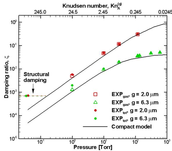
Figure 3. Comparison of predictions by the ESBGK-based compact model and experimental data in reference,<sup>14</sup>  $g_0 = [6.3, 2]\mu m$ ,  $b = 20\mu m$ ,  $t = [2.5, 2.25]\mu m$ ,  $L = 300\mu m$ .
