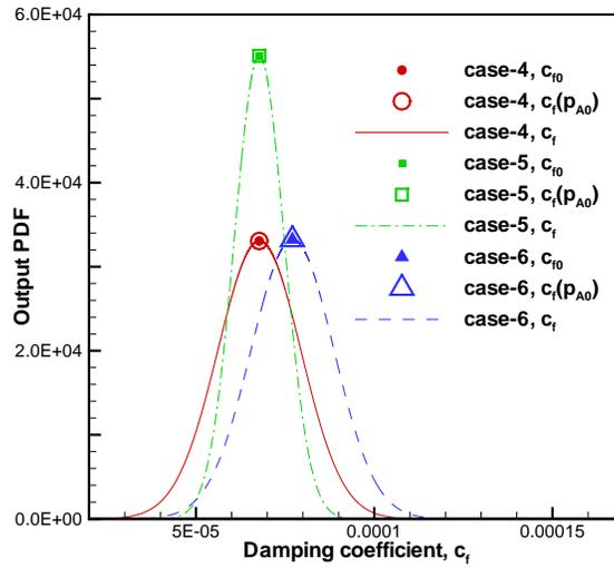
Figure 11. Output PDF of the damping coefficient due to uncertainties in the ambient pressure,  $g = 1.4\mu m$ .
