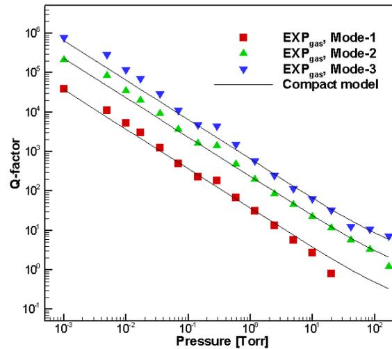
Figure 5. Comparisons of predictions by the ESBGK-based compact model and experimental data by Lee *et al*,<sup>16</sup>  $L = 500\mu m$ ,  $b = 18\mu m$ ,  $g_0 = 1.4\mu m$ ,  $t = 2.25\mu m$ ,  $\rho_s = 2.33e + 3 \text{ kg} \cdot \text{m}^{-3}$ ,  $E = 160GPa$ .
