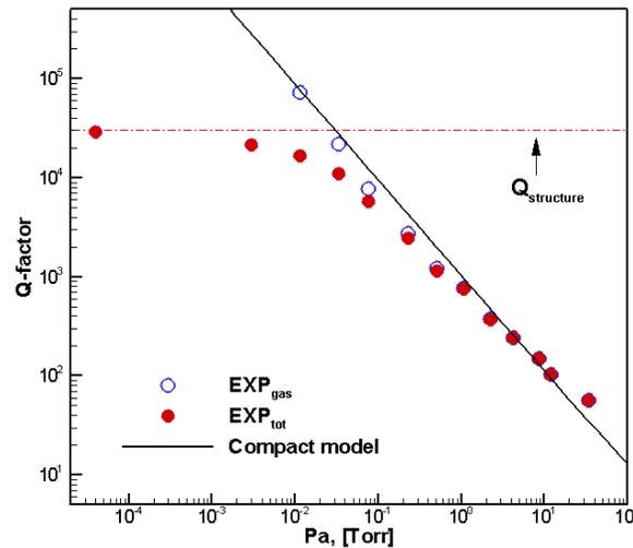
Figure 4. Comparison of predictions by the ESBGK-based compact model and experimental data in reference,<sup>15</sup>  $g_0 = 1.1\mu m$ ,  $b = 40\mu m$ ,  $t = 1.8\mu m$ ,  $L = 300\mu m$ .
