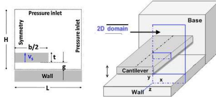
Figure 1. Schematic of computational domain and boundary conditions for squeeze-film damping simulations.
