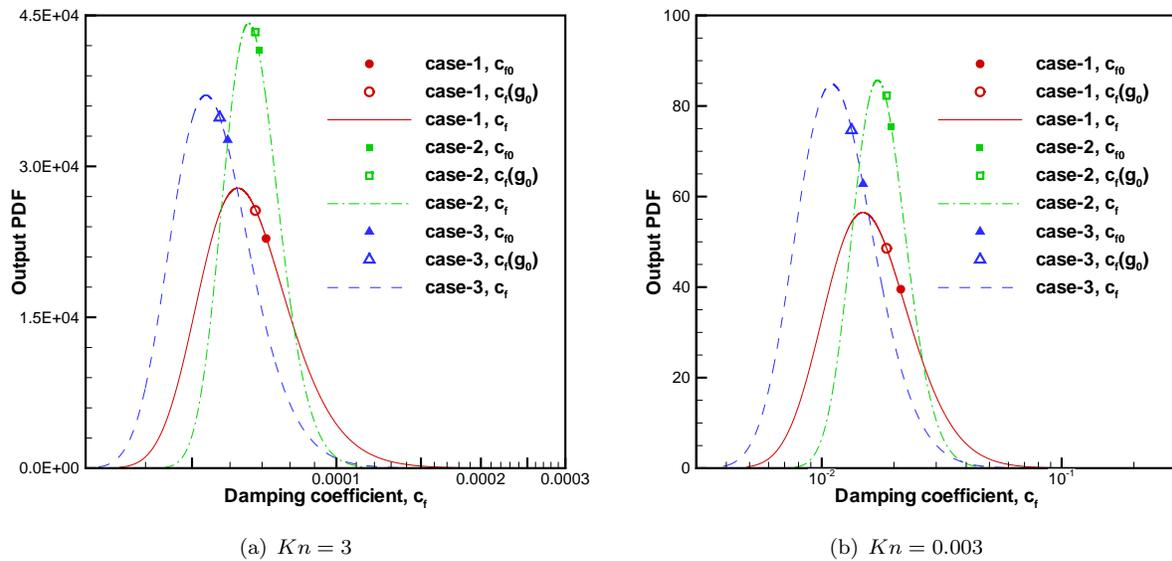
Figure 8. Output PDF of the damping coefficient due to uncertainties in the gap size.
