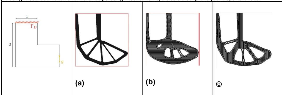
**Figure 2: case study of the L-beam and (a) optimal design in the case of a homogeneous bulk, (b) fabrication with crust of horizontal fiber infill, (c) crust and vertically oriented fiber infill**
