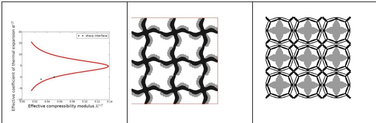
**Figure 1: on the left, optimum bound established by [6] the an effective isotropic material made of two constitutive phases and void, two predicted microstructure able to have a zero c.t.e with a threshold Young modules with two different operating mechanisms, a double strip one (centre) and a local**
