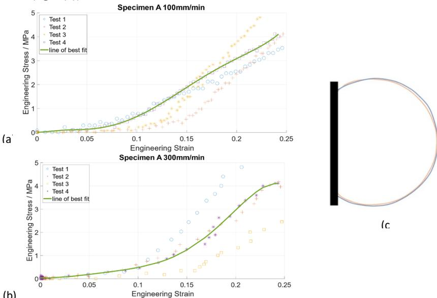
Fig 1: Uniaxial stress-strain data at (a) 100mm/min and, (b) 300mm/min crosshead speed (c) Schematic comparison showing maximum ball deformation during FE simulation (orange) and high-speed video analysis (blue) during impact at  $11.67\text{ms}^{-1}$ , inflated to 0.8bar.
