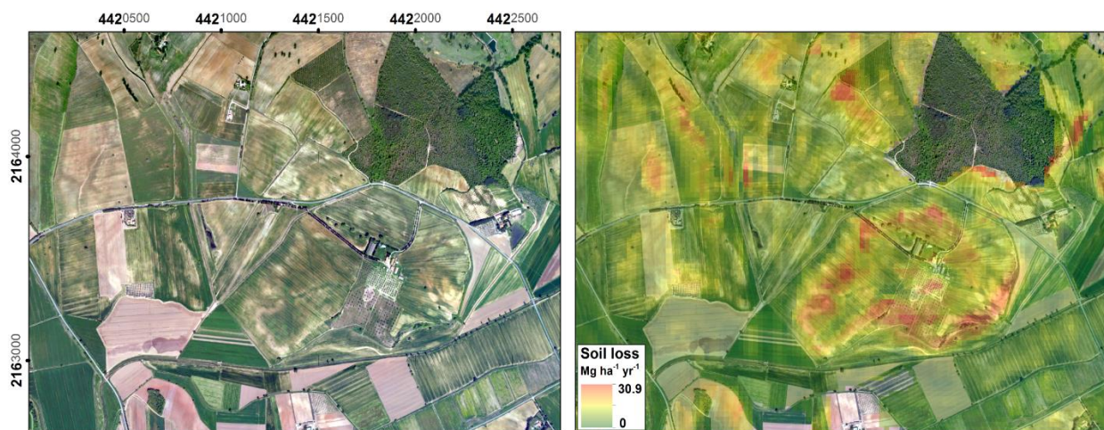
Figure 1. Example of the outcomes of RUSLE model applications in the Southern Tuscany (Magliano: 2163500E/4421500N).
