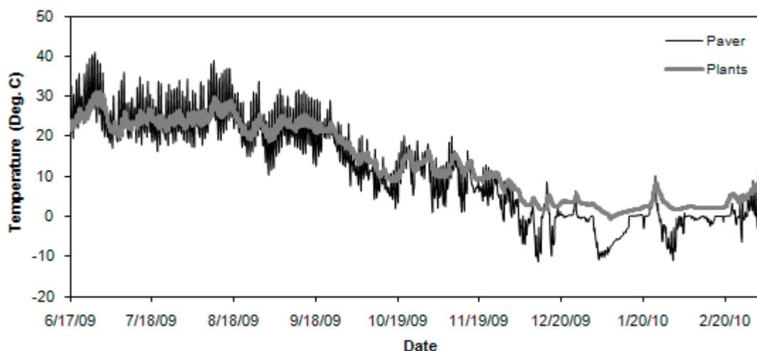
Figure 3: Surface temperature underneath reflective pavers and vegetation
