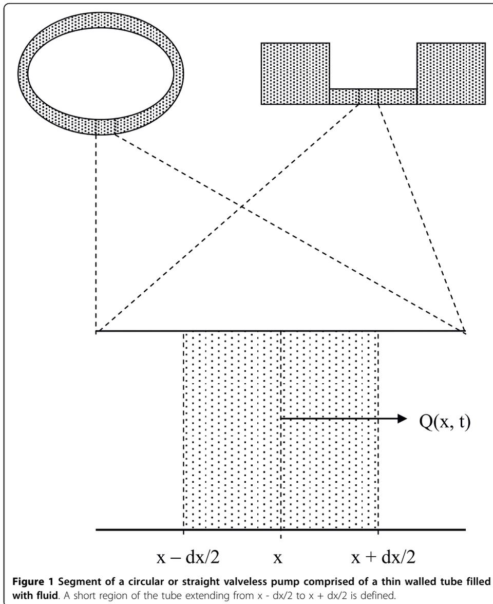
**Figure 1** Segment of a circular or straight valveless pump comprised of a thin walled tube filled with fluid. A short region of the tube extending from  $x - dx/2$  to  $x + dx/2$  is defined.
