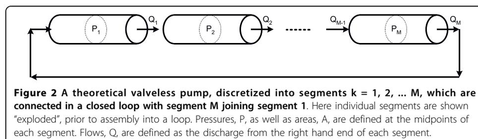
**Figure 2** A theoretical valveless pump, discretized into segments  $k = 1, 2, \dots, M$ , which are connected in a closed loop with segment M joining segment 1. Here individual segments are shown "exploded", prior to assembly into a loop. Pressures,  $P$ , as well as areas,  $A$ , are defined at the midpoints of each segment. Flows,  $Q$ , are defined as the discharge from the right hand end of each segment.
