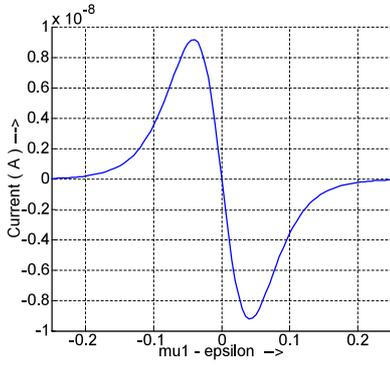
**Figure 7.3.** The thermoelectric current reverses direction from *p*-type ( $\mu_1 < 0$ ) to *n*-type ( $\mu_1 > 0$ ) samples.  $\gamma_1 = \gamma_2 = 0.005$  eV,  $k_B T_1 = 0.026$  eV and  $k_B T_2 = 0.025$  eV.
