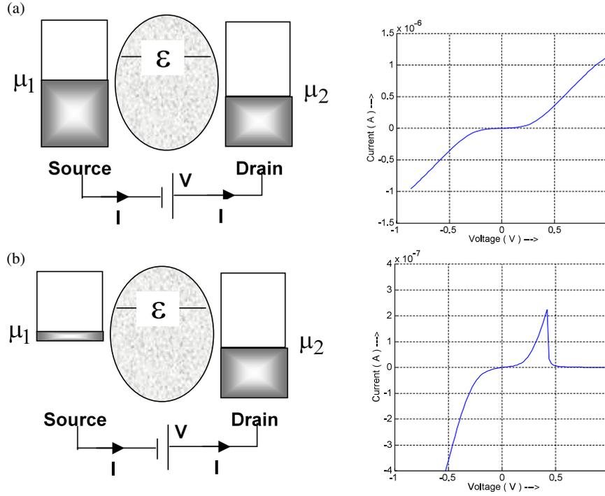
**Figure 7.1.** Current versus voltage calculated using equations (7.1)–(7.8) with  $\mu = 0$ ,  $\varepsilon = 0.2$  eV,  $V_G = 0$ ,  $k_B T = 0.025$  eV,  $U_0 = 0.25$  eV,  $C_D/C_E = 0.5$  and  $\gamma_1 = \gamma_2 = 0.005$  eV. The only difference between (a) and (b) is that in (a)  $\gamma_1$  is independent of energy, while in (b)  $\gamma$  is zero for energies less than zero. In either case  $\gamma_2$  is assumed to be independent of the energy.
