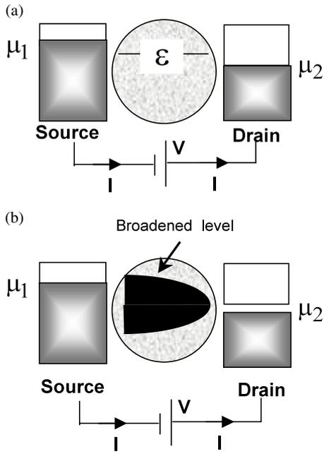
**Figure 4.1.** (a) A device with a small voltage applied across it causing a splitting of the source and drain electrochemical potentials  $\mu_1 > \epsilon > \mu_2$ . (b) The process of coupling to the device inevitably broadens it thereby spreading part of the energy level outside the energy range between  $\mu_1$  and  $\mu_2$  where current flows.
