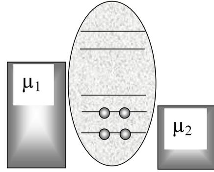
**Figure 3.1.** A positive voltage  $V_D$  applied to the drain with respect to the source lowers the electrochemical potential at the drain:  $\mu_2 = \mu_1 - qV_D$ . Source and drain contacts now attempt to impose different Fermi distributions as shown and the device goes into a state intermediate between the two.
