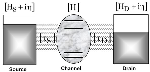
**Figure 8.2.** A channel connected to two contacts.
