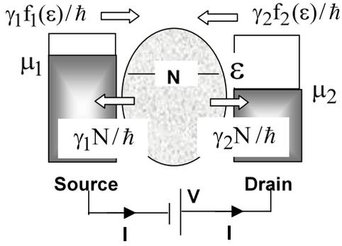
**Figure 3.2.** The flux of electrons into and out of a one-level device at the source and drain ends: the simple rate equation picture.
