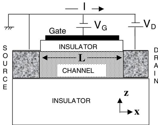
**Figure 2.1.** A sketch of a nanoscale field effect transistor. The insulator should be thick enough to ensure that no current flows into the gate terminal, but thin enough to ensure that the gate voltage can control the electron density in the channel.
