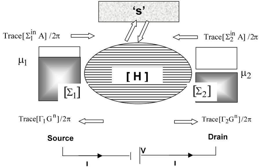
**Figure 8.1.** (See figure 7.6.) From numbers to matrices: the general matrix model, based on the NEGF formalism. Without the ‘s contact’ this model is equivalent to equation (6) of [12b]. The ‘s contact’ distributed throughout the channel describes incoherent scattering processes [12c]. In general this ‘contact’ cannot be described by a Fermi function unlike the real contacts.
