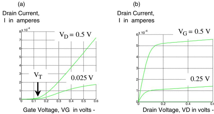
**Figure 7.5.** (a) The drain current ( $I$ ) as a function of the gate voltage ( $V_G$ ) for different values of the drain voltage ( $V_D$ ); (b) the drain current as a function of the drain voltage for different values of the gate voltage.
