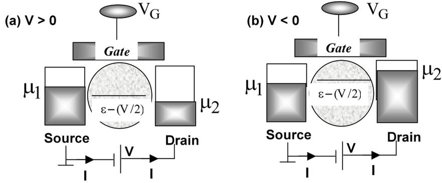
**Figure 5.1.** If the channel potential lies halfway between the source and drain potentials, significant current will flow for either bias polarity and the current–voltage characteristics will look symmetric.
