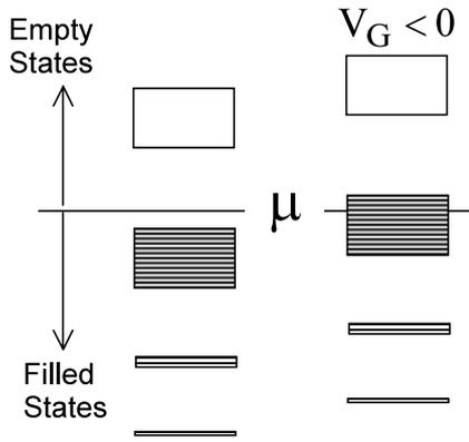
**Figure 2.3.** An example of p-type or hole conduction. A negative gate voltage ( $V_G < 0$ ) reduces the number of electrons in the channel. Nevertheless the channel will become more conductive once the electrochemical potential  $\mu$  is driven into the filled band since conduction depends on the availability of states around  $E = \mu$  and not on the total number of electrons.
