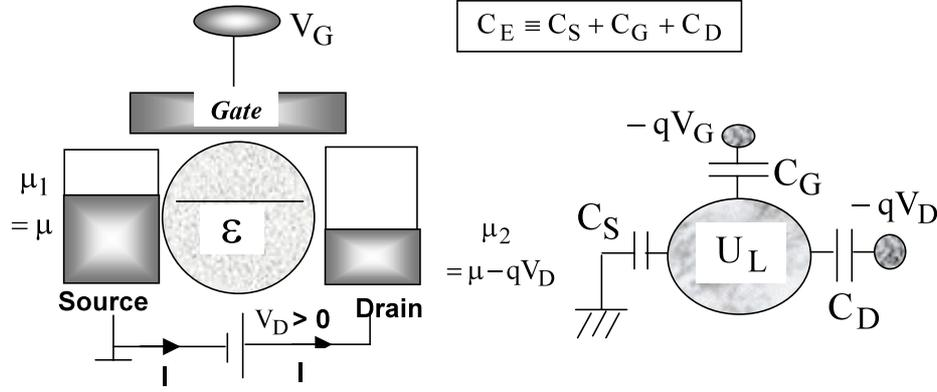
**Figure 5.3.** A simple capacitive circuit model for the ‘Laplace’ potential  $U_L$  of the active region in response to the external gate and drain voltages,  $V_G$  and  $V_D$ . The actual potential ‘ $U$ ’ can be different from  $U_L$  if there is a significant density of electronic states in the energy range around  $\mu_1$  and  $\mu_2$ . The total capacitance is denoted as  $C_E$ , where ‘ $E$ ’ stands for electrostatic.
