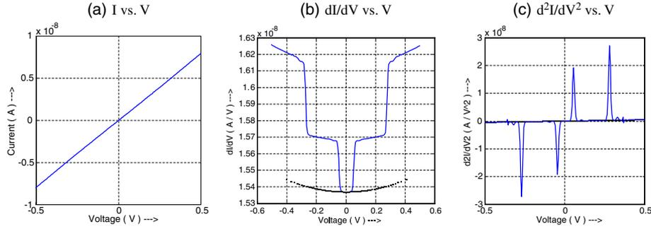
**Figure 7.7.** (a) Current ( $I$ ), (b) conductance ( $dI/dV$ ) and (c)  $d^2I/dV^2$  as a function of voltage calculated without phonon scattering (dashed line) and with scattering by phonons (solid curve) with two distinct frequencies having slightly different coupling strengths ( $D_1 = 0.5$ ,  $\hbar\omega_1 = 0.075$  eV and  $D_2 = 0.7$ ,  $\hbar\omega_2 = 0.275$  eV).
