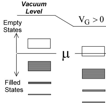
**Figure 2.2.** Allowed energy levels that can be occupied by electrons in the active region of the device such as the channel in figure 2.1. A positive gate voltage  $V_G$  moves the energy levels down while the electrochemical potential  $\mu$  is fixed by the source and drain contacts which are assumed to be in equilibrium with each other ( $V_D = 0$ ).
