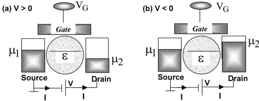
**Figure 5.2.** If the channel potential is tied to the source and unaffected by the drain potential, significant current will flow (a) for  $V > 0$ , but not (b) for  $V < 0$ , making the current–voltage characteristics look rectifying.
