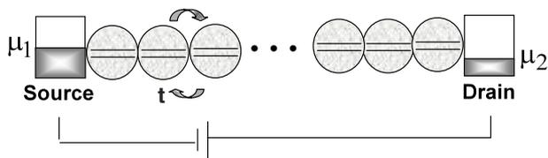
**Figure 9.1.** A large conductor can be viewed as an array of unit cells. If the conductor is extended in the transverse plane, we should view each unit cell as representing an array of unit cells in the transverse direction.
