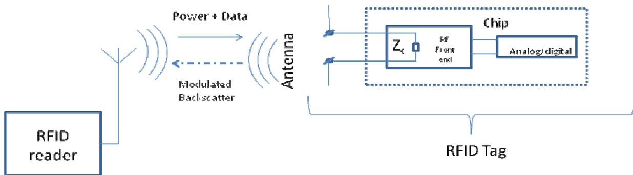
Figure 8. Passive RFID system (Lam, Nikitin & Rao, 2006)
