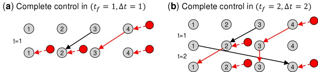
FIG. 2. Controlling the simple temporal network illustrated in Fig. 1. The driver nodes and independent time-respecting paths are marked with the red colors. (a) Three driver nodes are required to reach full control over interval  $t = 1$ . (b) Two driver nodes are needed to reach control over interval  $t = 2$  as the self-loop of *node 3* at the interval  $t = 2$  enables controlling *node 3* through *node 4*.
