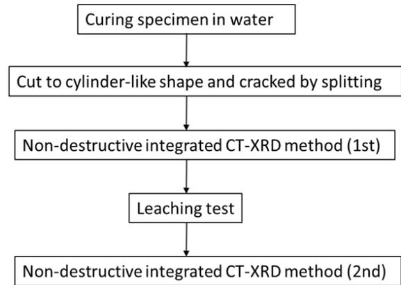
Figure 5. Flowchart of measurements.
