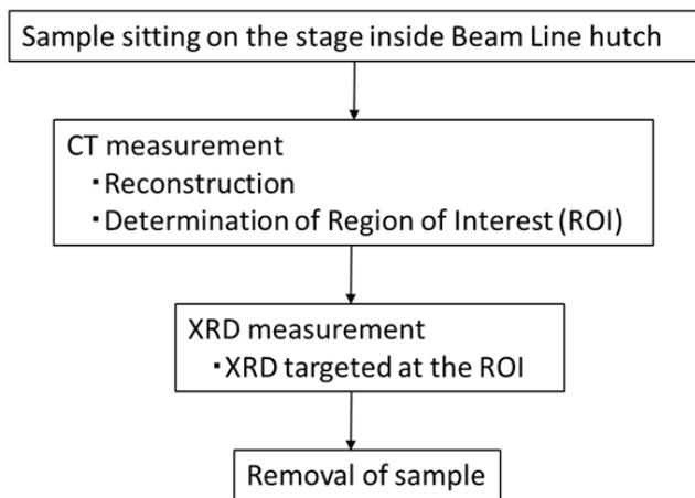
Figure 1. Flowchart of nondestructive integrated CT-XRD method.
