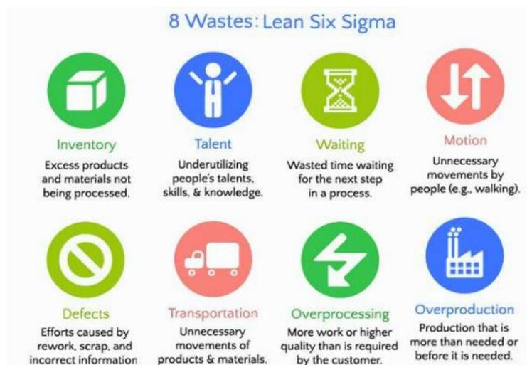
Figure 1: Common wastes identified by lean six sigma (Upkar, R.S., Lande, M.S. and Jawalekar, S.B., 2016)
