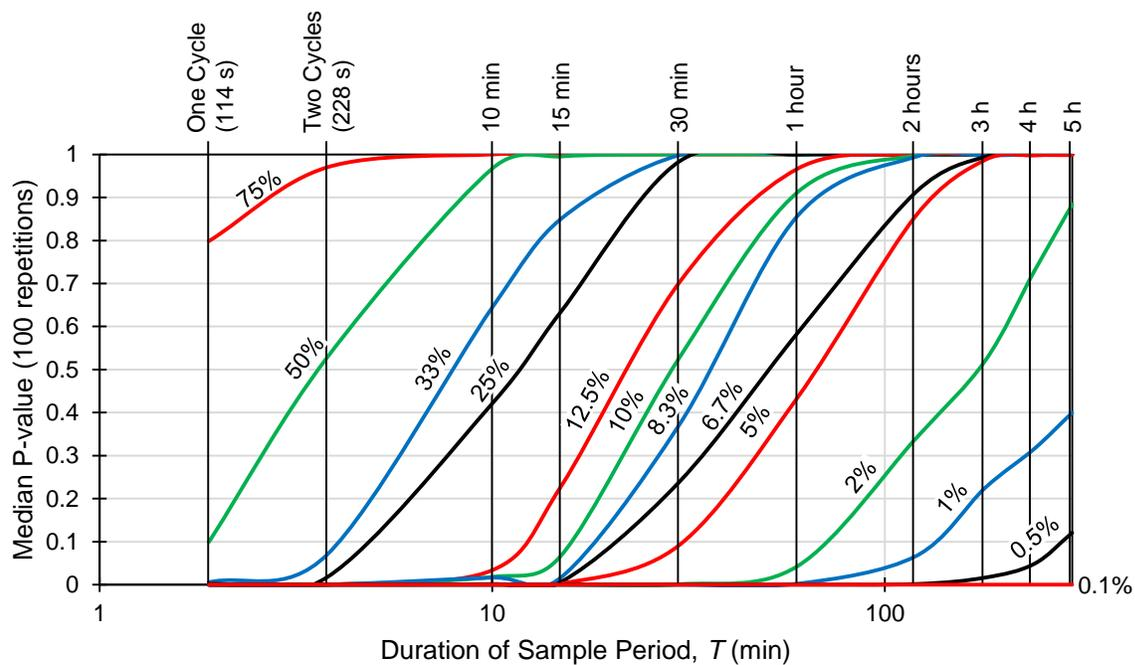
Figure 4. Relationship between analysis period  $T$  and the quality of arrival profile estimation (average  $P$ -value from KS tests for 100 separate random samples) at various values of market penetrations,  $p$ . The percentage displayed on each curve shows the value of  $p$ .
