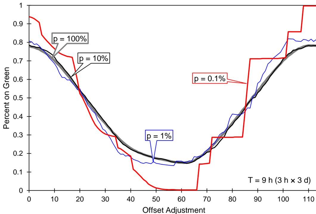
Figure 8. Impact of layering multiple days of data: Offset-performance data for three aggregated days of data (9 hours total), at different levels of  $p$ .
