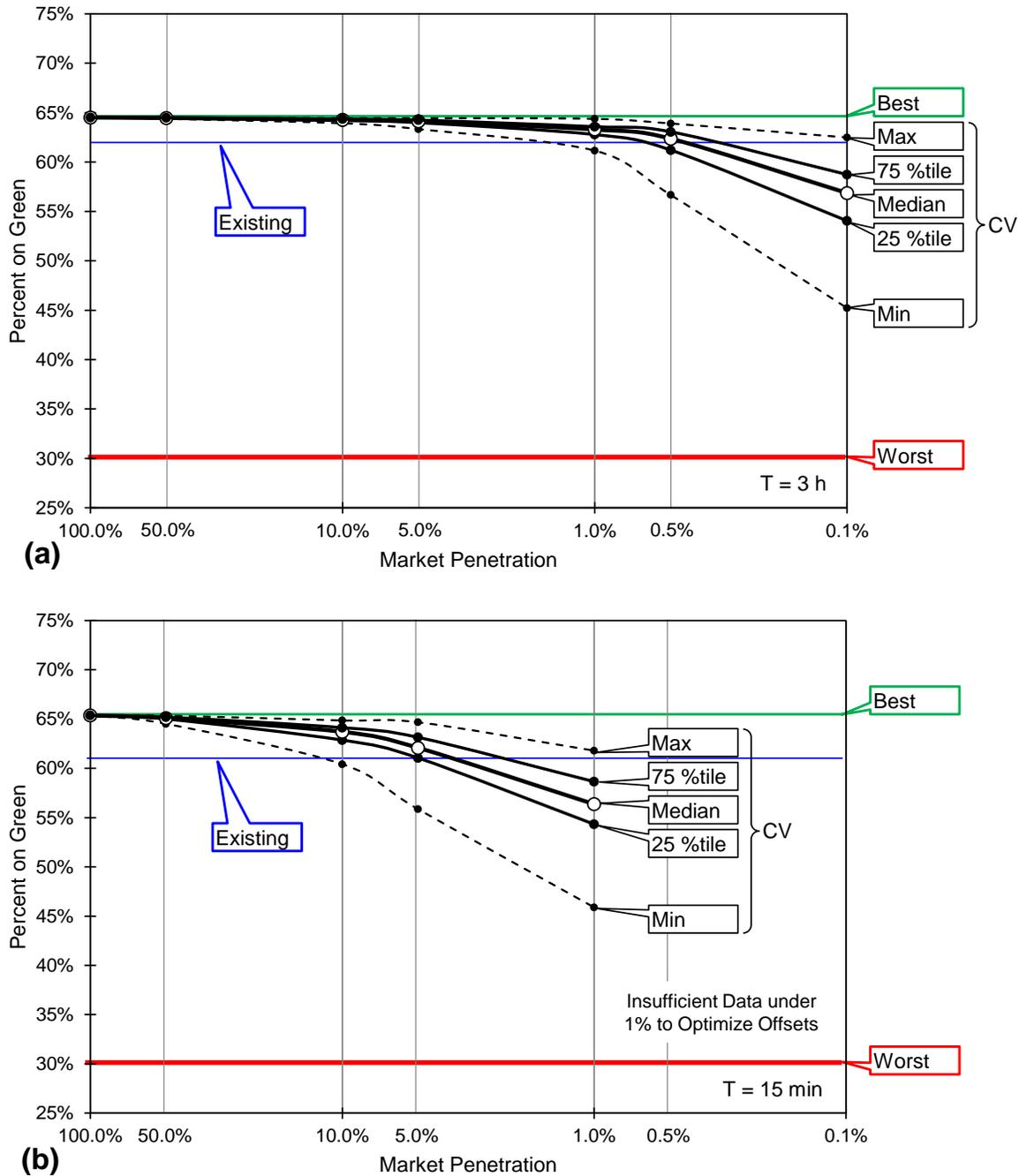
Figure 7. Sensitivity of optimization outcome to market penetration  $p$  for (a)  $T = 3$  h and (b)  $T = 15$  min. Lines marked “CV” show the distribution of results for 100 iterations at each trial value of  $p$ .
