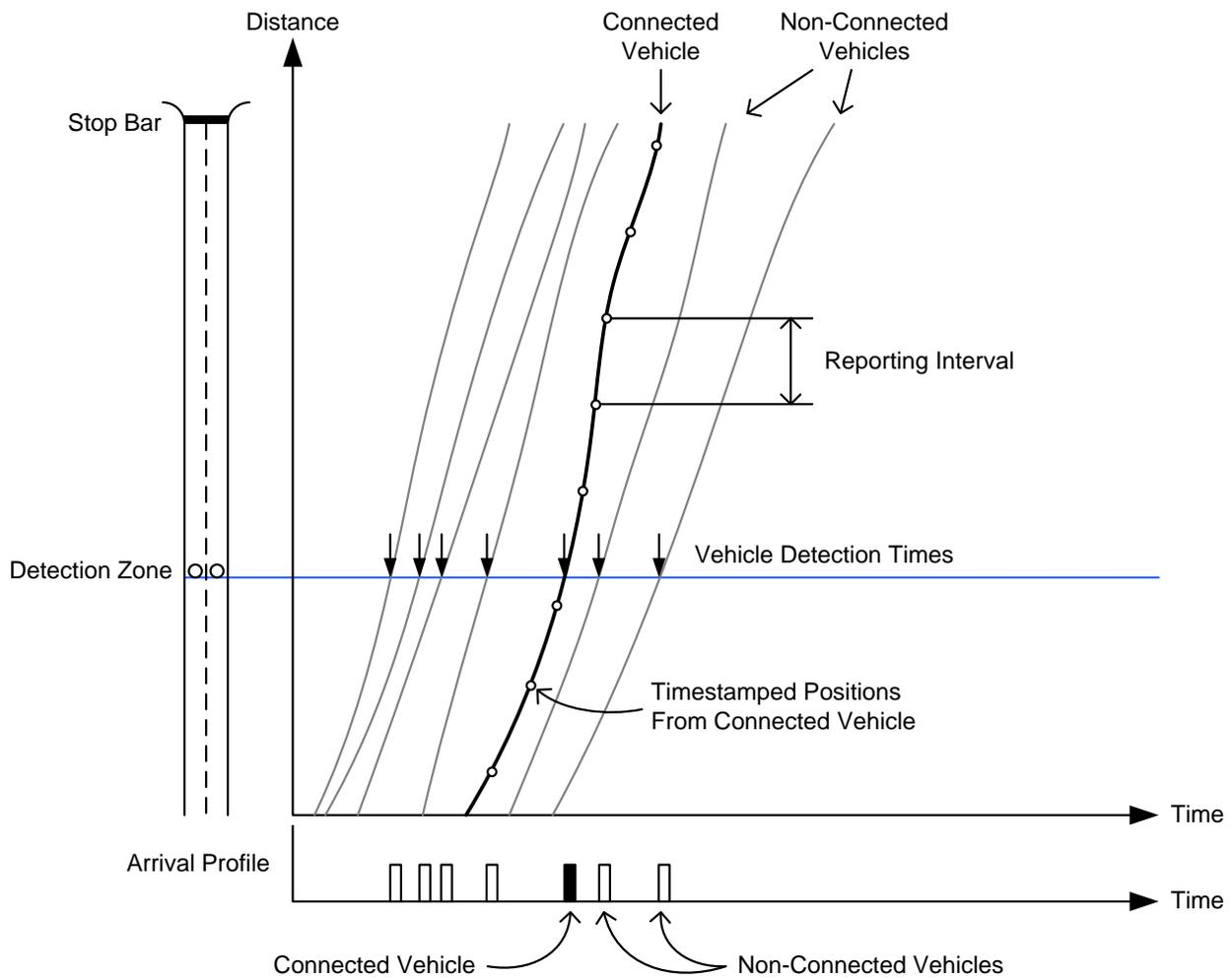
Figure 2. Traditional vehicle arrival measurement with detection, and opportunities for detector-free measurement using connected vehicle data.
