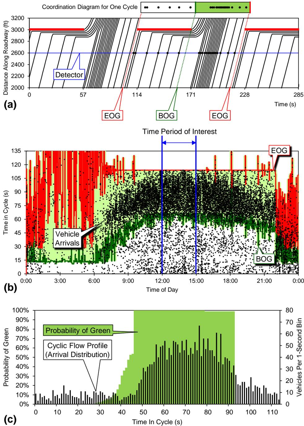
Figure 1. Three graphical representations of vehicle arrival and phase status data based on conventional (complete) detection: (a) a time-space diagram, and a coordination diagram for one cycle; (b) a Purdue Coordination Diagram (PCD) covering 24 hours; (c) a cyclic flow profile showing arrival and probability of green distributions.
