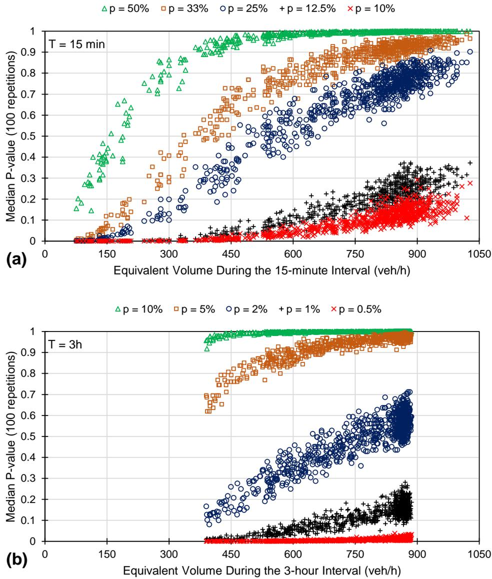
Figure 5. Relationship between traffic volume and the quality of arrival profile estimation. Each point is the average  $P$ -value of KS tests for 100 separate random samples for a different starting time. Data shown for (a)  $T = 15$  min; and (b)  $T = 3$  h.
