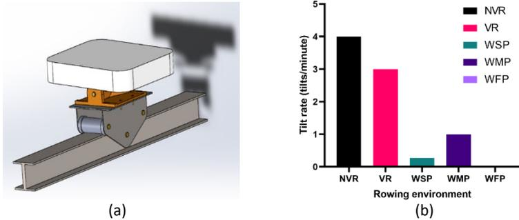
Fig. 1: (a) Design of the mediolateral axis between the seat frame and the seat to allow mediolateral movement, (b) Tilt rate for an elite rower in different rowing environments.
