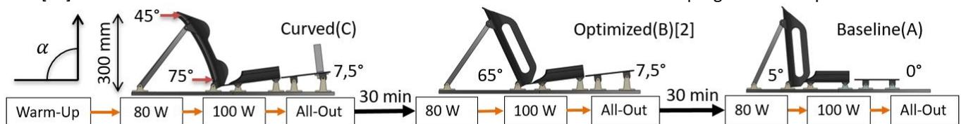
Fig. 1: Experimental design for evaluating and comparing the performance of the three different chair designs.
