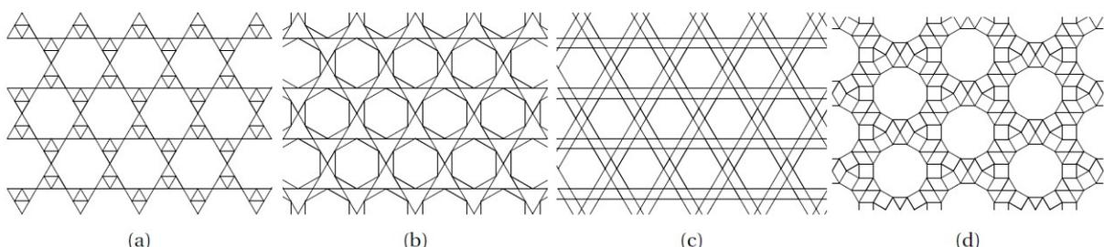
Fig 1. Lattice micro-architectures investigated: (a) Kagome with concentric triangles (KT), (b) Kagome with concentric hexagons (KH), (c) Double Kagome (DK) and (d) the 'modified dodecagonal structure' (MD).
