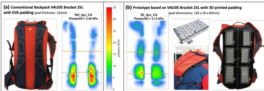
Fig. 1: View of the back panel padding and exemplary mean pressure distribution images for (a) conventional VAUDE Bracket 25L and (b) prototype with 3D printed padding.
