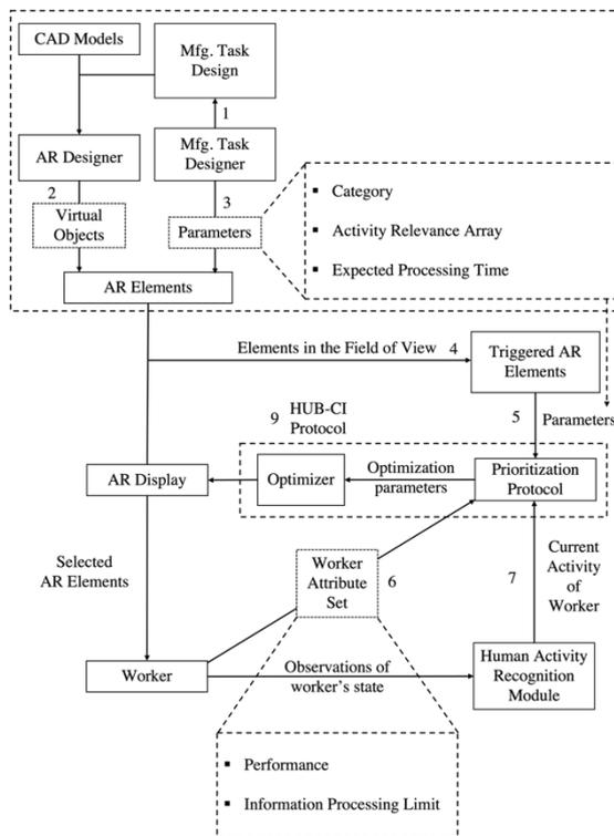
Figure 1: AR design framework with HUB-CI protocol.
