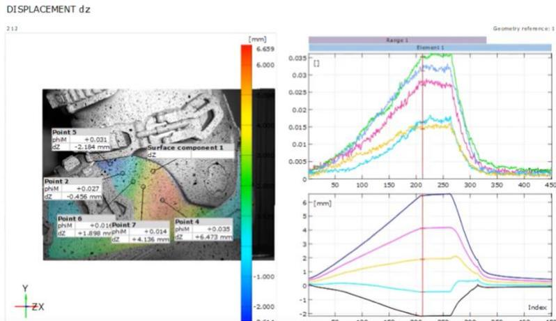
Figure 2: example of DIC analysis for the validation of the FEM model.
