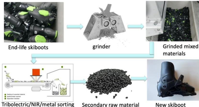
Fig. 1: scheme of the process for recycling of ski-boots
