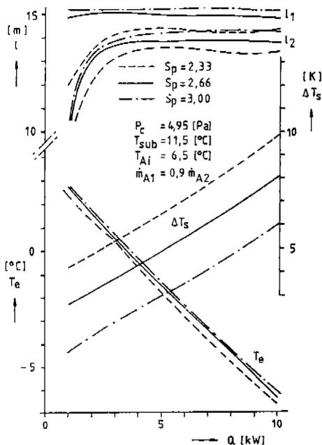
figure 4. Evaporation temperature and length of the two series of evaporation regions and superheat as a function of the heat load. Simulation results of an evaporator with a conventional TEV for three different setpoints.
