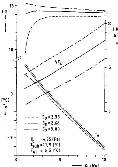
figure 3. Evaporation temperature and length of the evaporation region and superheat as a function of the heat load. Simulation results of an evaporator with a conventional TEV for three different setpoints.
