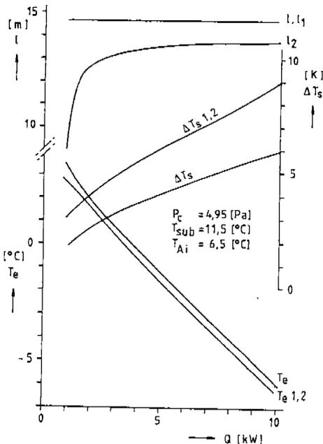
figure 5. Evaporation temperature, length of the evaporation region(s) and superheat as a function of the heat load. With and without uniform refrigerant and air flow along the evaporator pipes. Simulation results of an evaporator controlled in such a way that the length of the (shortest) superheat region is kept at a constant value of 0.6 m.
