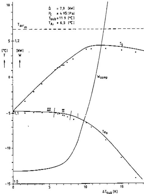
figure 6. Saturation and vapour temperature at the outlet of the evaporator measured (points) and simulated (lines), and the calculated compressor work, necessary to keep the heat load constant, as a function of the superheat.
