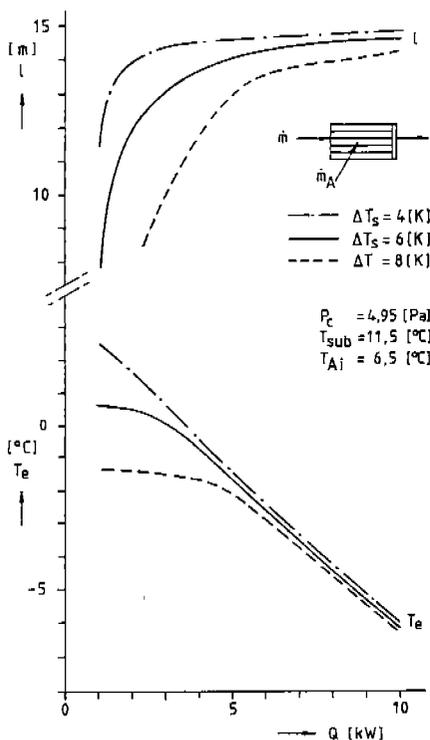
figure 1. Evaporation temperature and length of the evaporation region as a function of the heat load. Simulation results of an evaporator with a TEV with integrative action for three different setpoints.
