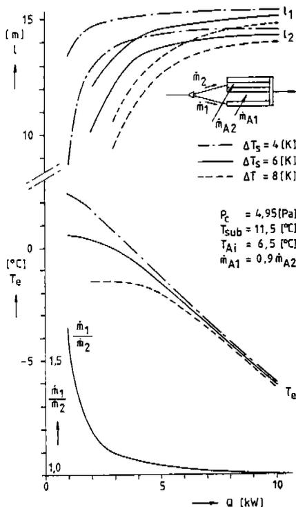
figure 2. Evaporation temperature and length of the two series of evaporation regions and, for the case of 4 K superheat, the ratio of the refrigerant massflows as a function of the heat load. Simulation results of an evaporator with a TEV with integrative action for three different setpoints.
