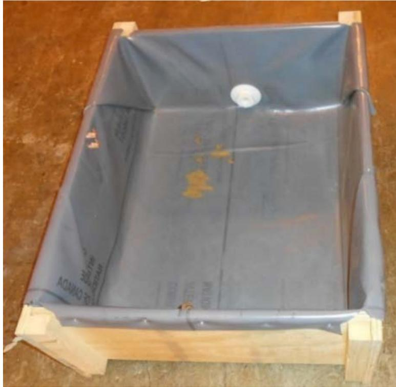
*Figure 2 - Virtual pig constant temperature heat source for testing apparatus.*
