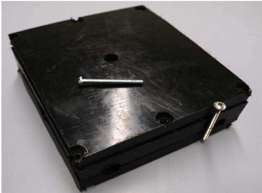
*Figure 4 - This is the assembled box, which has a lid attachment consisting of only four screws, with an additional two screws to attach the overall box to the farrowing crate framework.*
