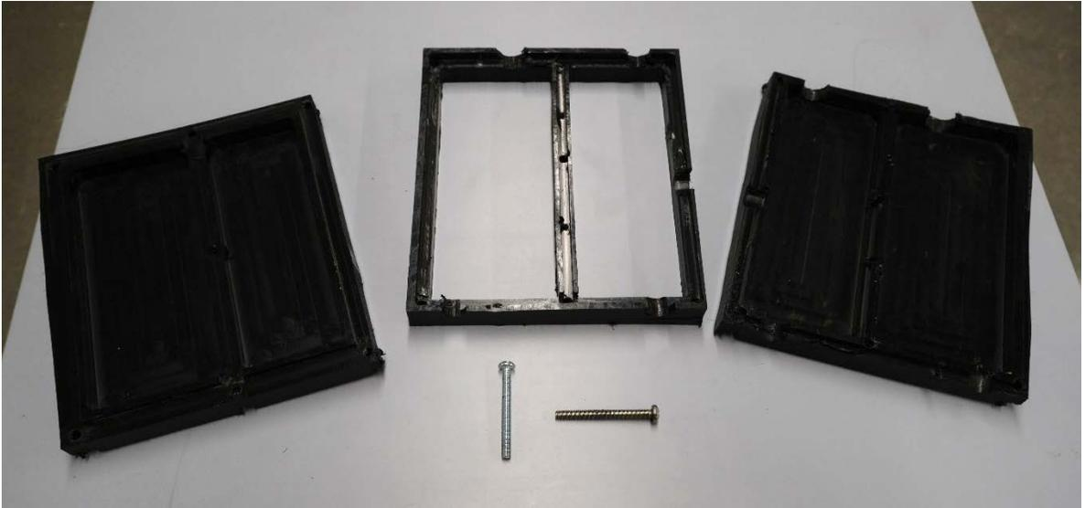
*Figure 3 - This is the redesigned three-piece control box, with the lid on the left, the riser in the middle, and the base on the right. The riser has six holes to attach to the base and hold the components internally. These pieces are designed for simple alignment with tongue and groove joints. There is a longer attachment side on the edge with the flow control valve.*
