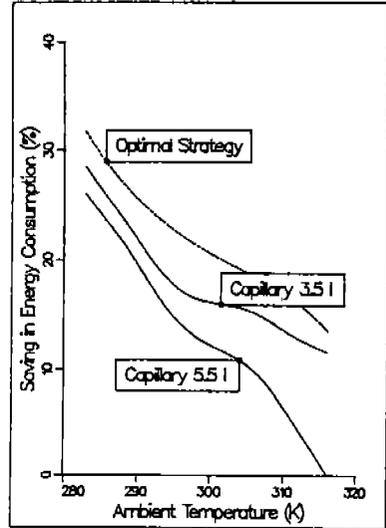
Fig. 10 Saving in energy consumption -in comparison with an on/off controlled cycle- possible with an optimally controlled expansion element and charge, and with a capillary of 5.5 l capacity. Values obtainable by the application of the 3.5 l capillary and a fixed charge (113 g) are given as well.
