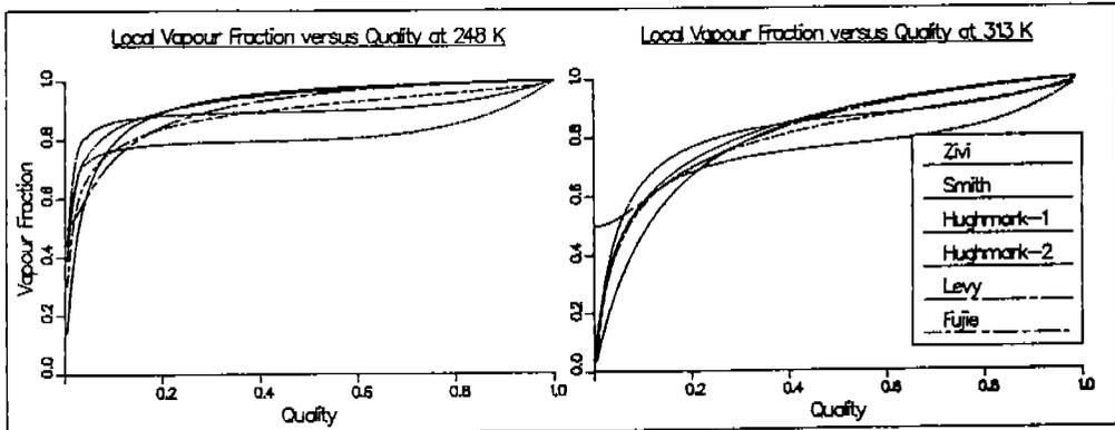
Fig. 1 Local void (vapour) fraction as a function of the quality (for typical evaporation and condensation temperatures of 248K and 313K, respectively), determined by the use of various kinds of correlation functions -for the relationship recommended by Hughmark /9/ two curves are given, representing the minimum and maximum values being realistic for the heat exchangers investigated in this contribution-
