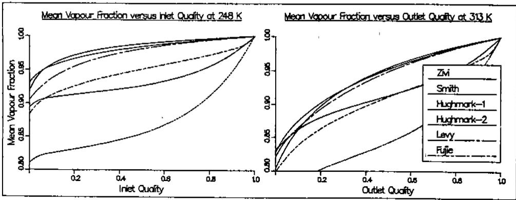
Fig. 2 Mean void fraction as a function of the inlet quality (or outlet quality in the case of the condenser) for the temperatures, equal as in Fig. 1; this mean fraction is determined for a dry evaporator (or a subcooled condenser, i.e. integration has been performed from inlet quality to 1.0. -for the relationship of Hughmark /9/ the same statements as given under Fig. 1 are valid-
