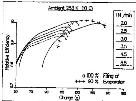
Fig. 6 Influence of the capillary tube capacity on the efficiency of the cycle -in relative sense-, as a function of the refrigerant charge applied. Ambient temperature 283K (10 C).
