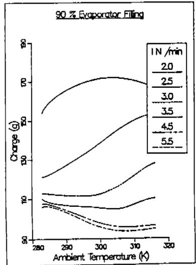
Fig. 9 Charges of refrigerant, the application of which results in a "90% liquid filling grade" (i.e. 90% of the heat exchanger tubing is in contact with evaporating liquid) of the evaporator. The charge necessary is given as a function of the ambient temperature for a number of capillary tube capacities (from 2.0 to 5.5 l).
