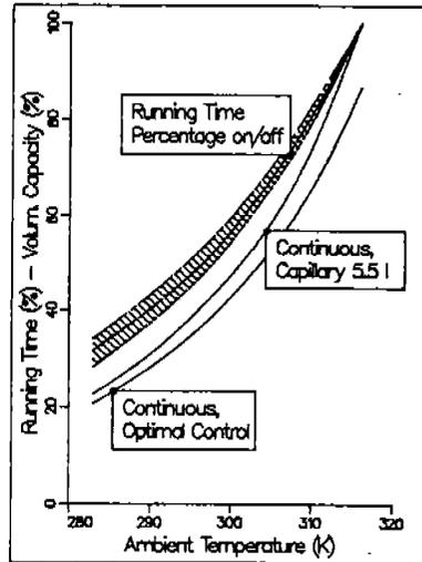
Fig.5 Running time percentage and volumetric capacity of the on/off and continuously controlled systems (normalized to 100% at an ambient of 316K) for
