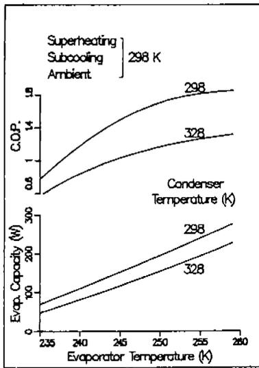
Fig.3 Capacity and COP of the -commercially available- compressor applied in the 330 l freezer investigated. Subcooling, superheat and ambient temperature amount to 298K (25 C)
