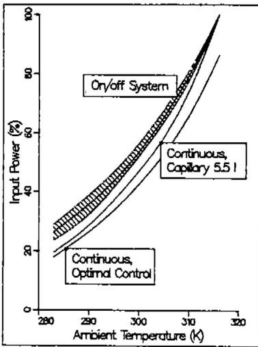
Fig. 4 Energy consumption dependent on the ambient temperature, in relative sense (normalized to 100% at an ambient of 316K (43 C) where continuous running is assumed) for
