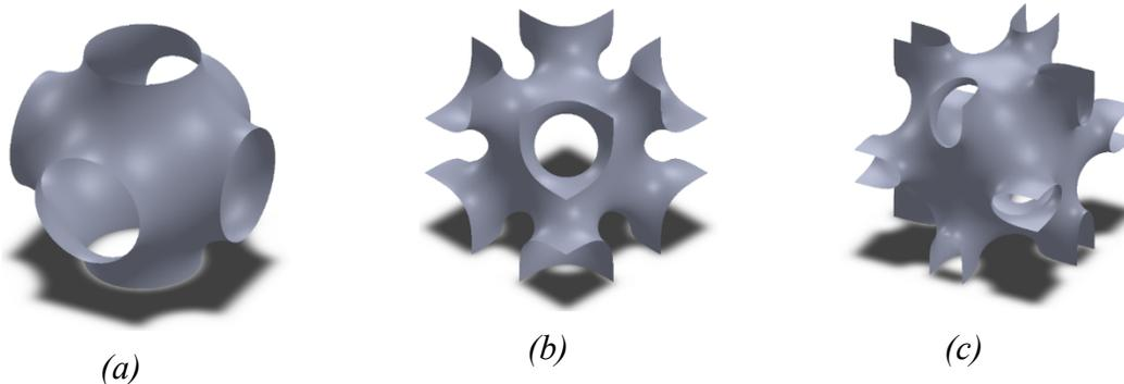
Figure 1: TPMS surfaces: (a) Schwarz Primitive surface, (b) Schoen IWP surface, and (c) Neovius surface.
