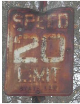
(a) Speed limit sign beyond the end of useful life.
