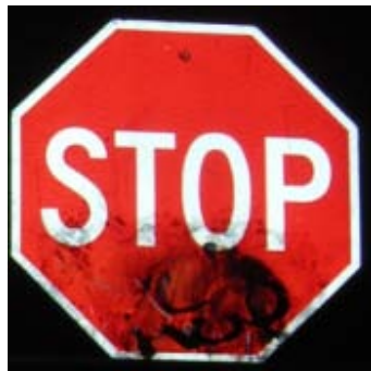
(f) Damage from graffiti cleaning solvent.
