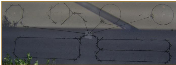
Loop detector test bed.
