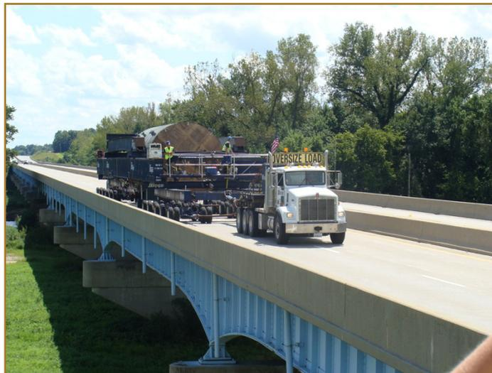
Beam and dolly transporter for superload test
