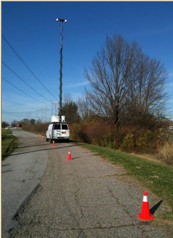
Exterior setup of the Mobile Traffic Laboratory
