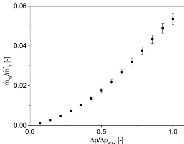
Figure 5: Secondary leakage in the valve system D1.
