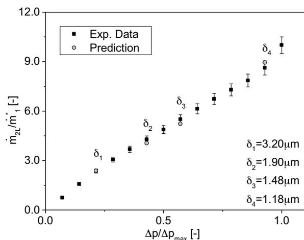
Figure 6: Leakage in the valve system D2.
