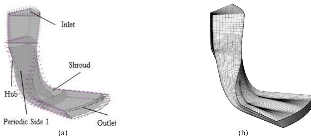
**Figure 2:** Fluid flow blade passage with the boundary conditions (a) and structural meshing of the fluid flow passage (b)
