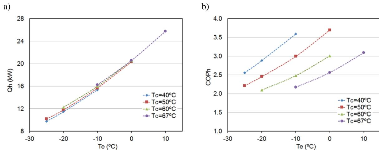
**Figure 7:** a) Heating capacity as a function of evaporating temperature. b) Heating COP as a function of evaporating temperature at several condensing temperatures
